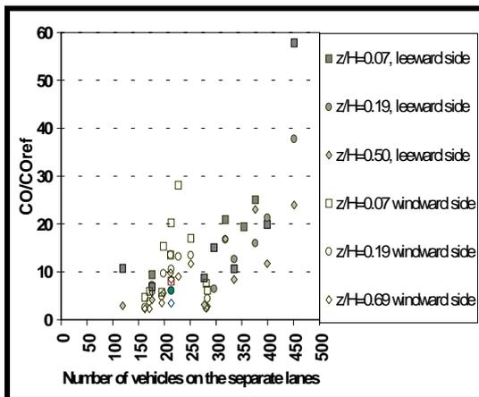
Figure 2.5 Dependence of CO concentration on the number of vehicles
