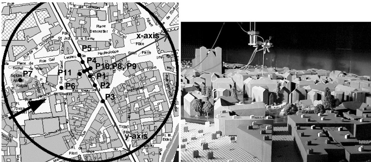
Fig. 2.1: Area in the center of Nantes reconstructed in the wind tunnel model (circle) with the profile locations (left) and photo of the model installed in the boundary layer wind tunnel (right).
