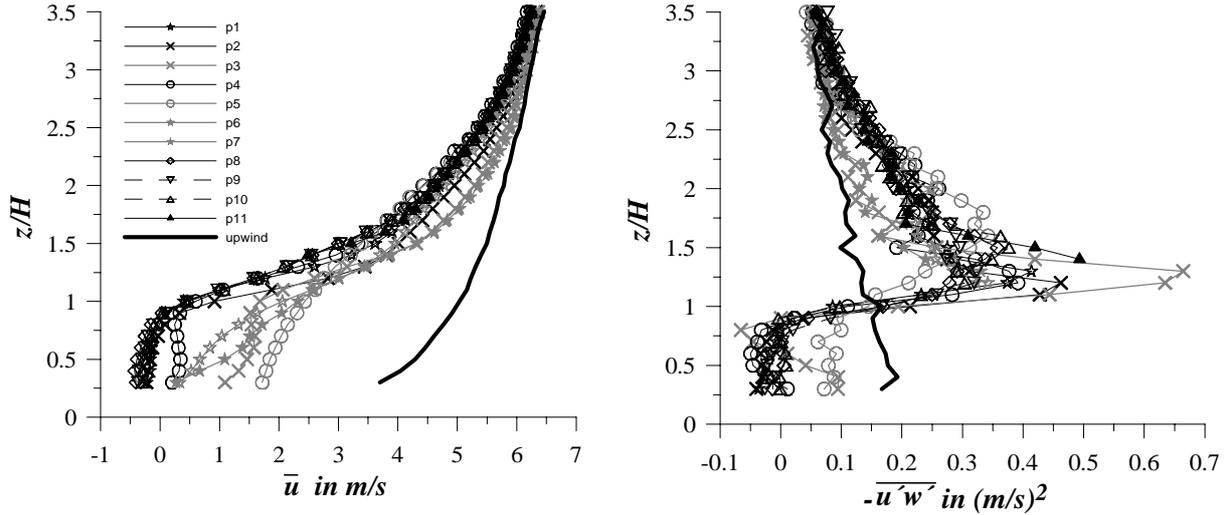
Fig. 3.1: Mean wind (left plot) and shear stress (right plot) profiles measured at the 11 sampling locations (see text for details)
