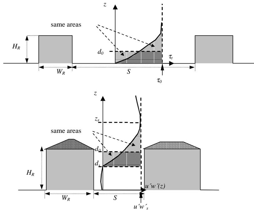
Fig. 4.2: Determination of displacement height  $d_0$  according to the integral condition proposed by Jackson (1981). The upper sketch shows the application to a situation with low building density, the lower one to an urban street canyon configuration with weak momentum flux inside the canopy.
