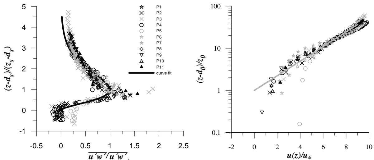
Fig. 4.1: Left panel: Scaling of measured shear stress profiles. Right panel: Comparison of measured mean wind profiles with a logarithmic profile. See text for more details
