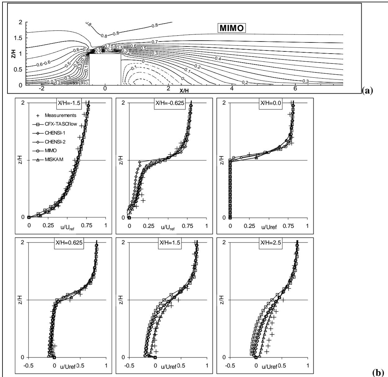
**Figure 2.2.2:** (a) Vertical cross section of the dimensionless  $u$ -component predicted by MIMO in the centre plane of the flow, (b) Comparison of the dimensionless profile of the  $u$ -component measured and predicted by the models in the centre plane of the flow at various distances.
