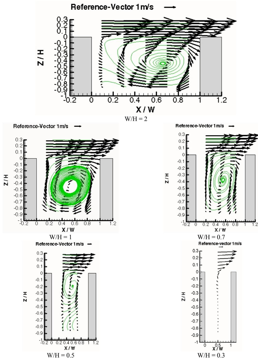
Figure 3b: Variation with aspect ratio ( $W/H$ ) of the flow pattern in a 2-D canyon (WT experiments – 2d cavity)
