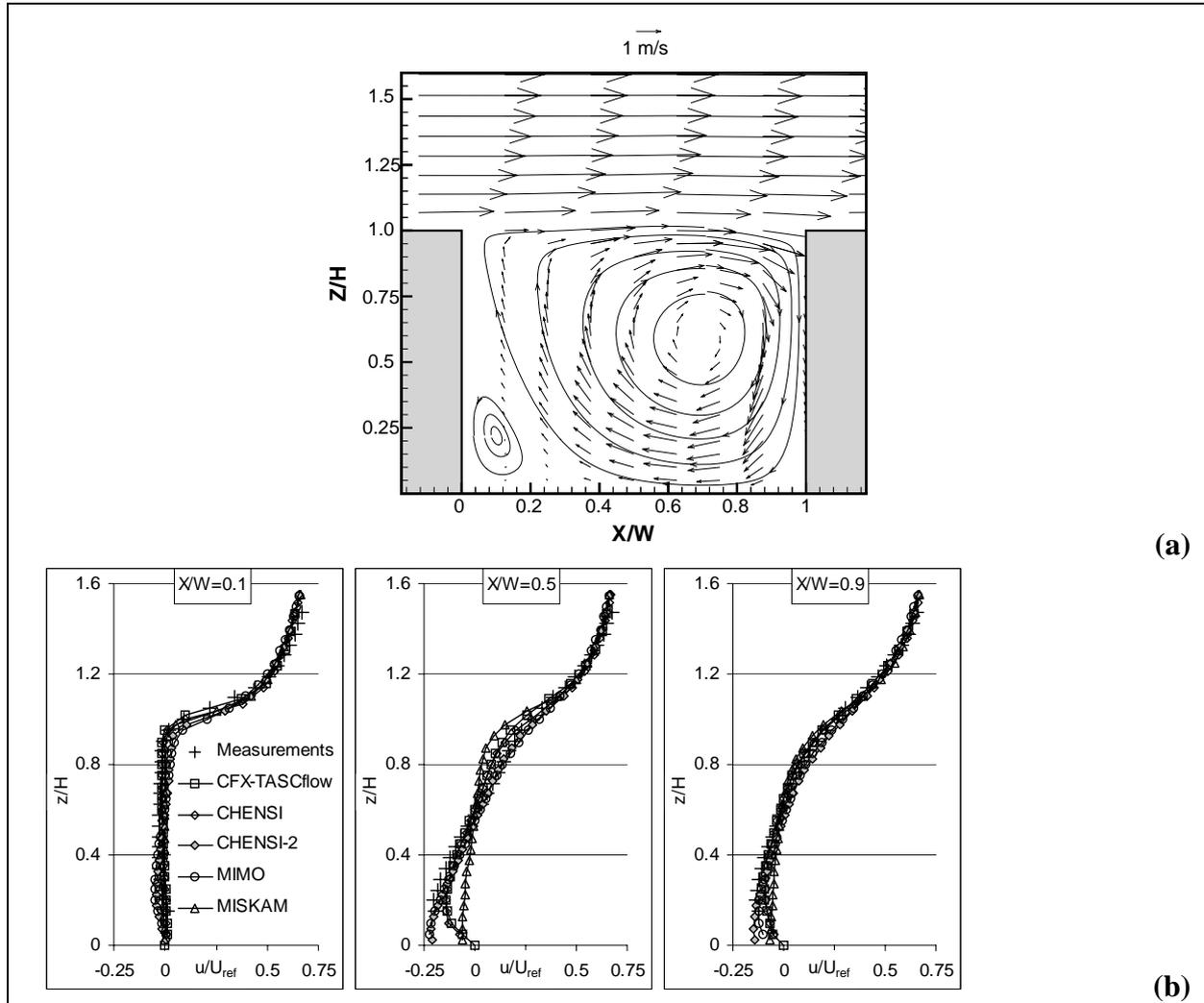
**Figure 2.2.1:** (a) The flow field within and above the cavity as it was reproduced by CHENSI, (b) Comparison of the profile of the  $u$ -component observed in the wind tunnel with that predicted by the numerical models at  $X/W=0.1, 0.5,$  and  $0.9$ .
