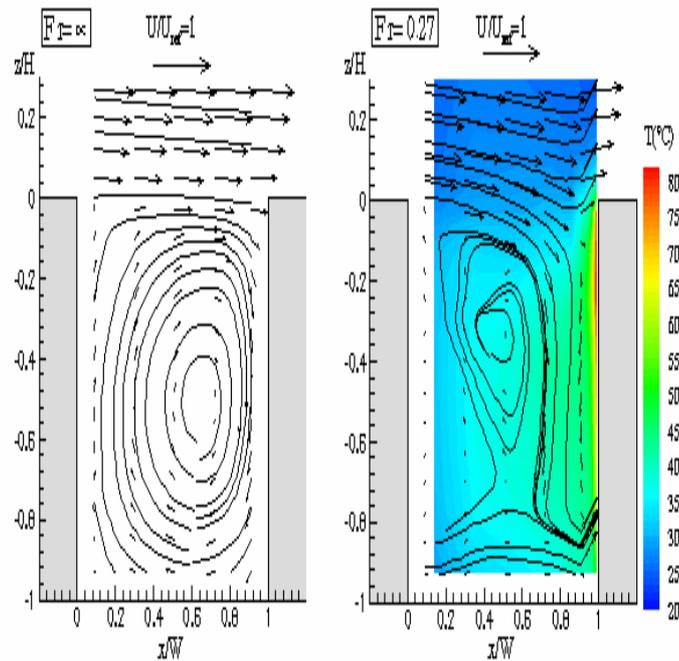
Figure 6: Projected mean velocity vectors, mean temperature contours and streampaths on canyon centre-plane. Left: Neutral case,  $U_{ref}=1\text{m/s}$ , Right:  $Fr=0.27$ ,  $U_{ref}=0.5\text{m/s}$ ,  $T_w=120^\circ\text{C}$
