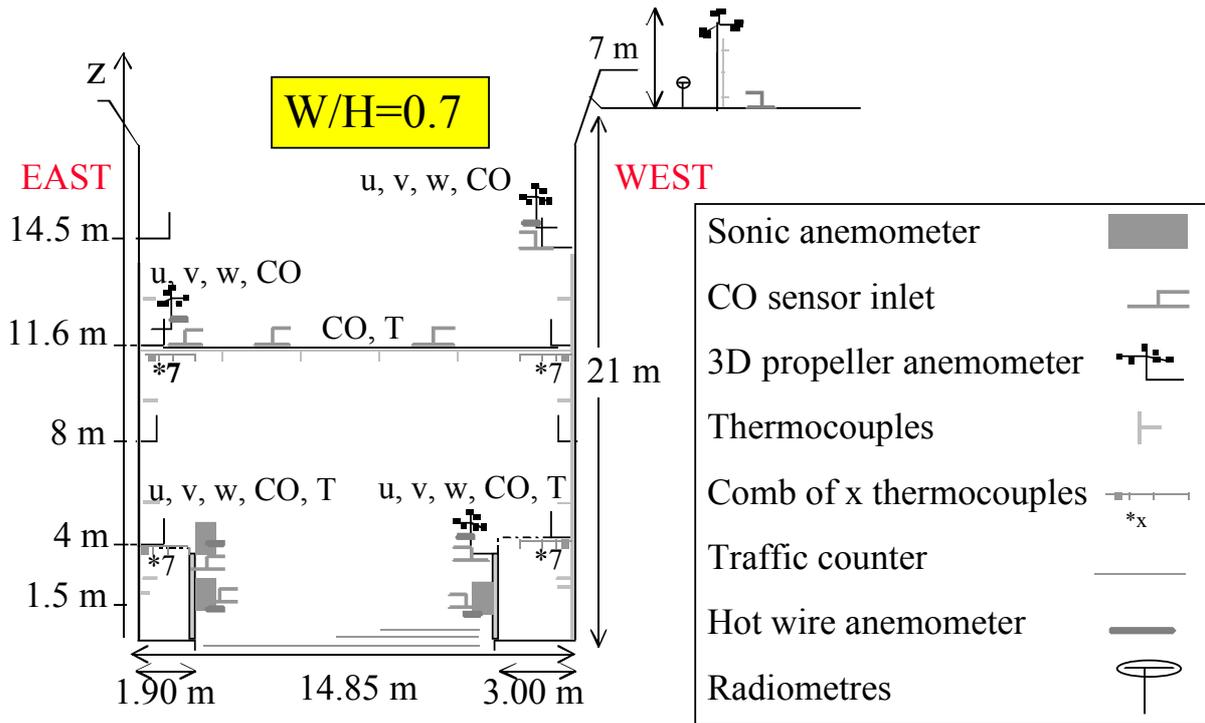
Figure 1: Schematic representation of the measurement site and instruments involved.
