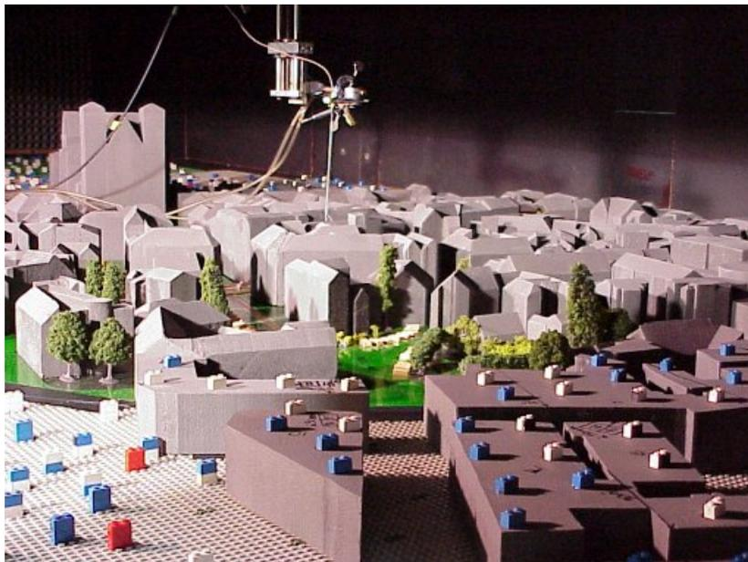
Figure 2: Wind tunnel model of 'Rue de Strasbourg' in Nantes and its surroundings
