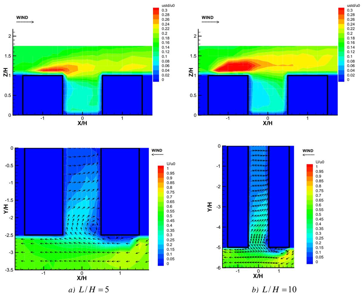
Figure 5: Influence of span wise aspect ratio  $L/H$  on the flow field inside an isolated 3D street canyon configuration.
