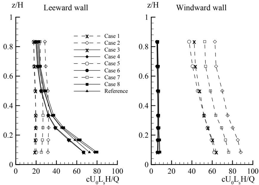
Figure 7: Non-dimensional concentration profiles on leeward and windward walls for different roof shapes (Table 1) when considering either the leeward or windward roof.
