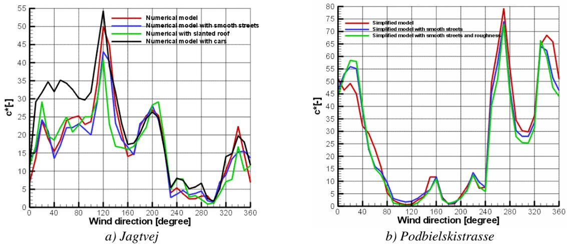
Figure 8: Influence of small-scale geometry simplifications on dimensionless concentrations as a function of wind direction for two different street canyon configurations
