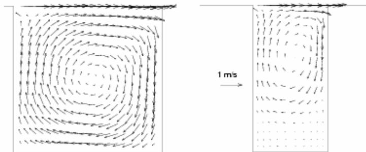
Figure 2: Velocity fields for two street canyon configurations as predicted with CFX-TASCflow.
