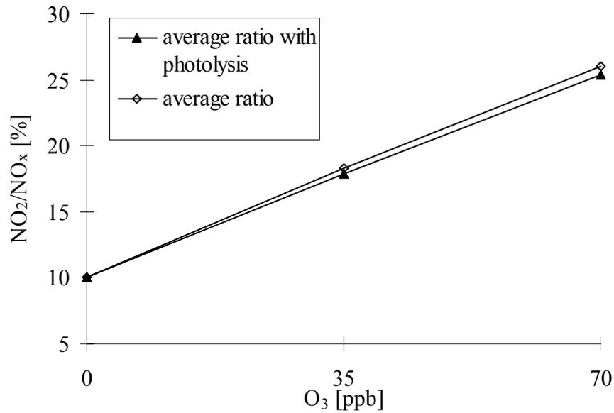
Figure 4: Predicted NO<sub>2</sub>/NO<sub>x</sub> ratio for various background ozone levels.
