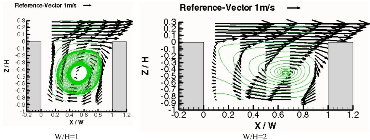
Figure 1: Flow patterns inside 2D cavities for different aspect ratios.
