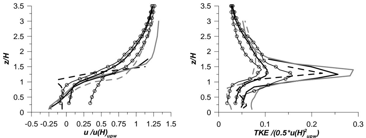
Figure 10: Averaged profiles of the u-velocity component (left plot) and turbulence kinetic energy profiles (right plot). Black lines: Idealised canyon UKA-WT, solid for flat roofs and dashed for slanted upwind roof. Grey lines: Idealised canyon -EPA-WT, solid for first canyon and dashed for sixth canyon. Circles: Rue de Strasbourg-UKA-WT (thick line - mean; thin lines - lowest/highest values).
