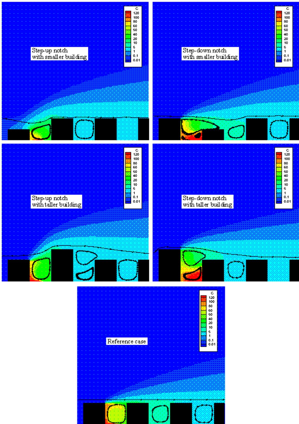
Figure 5: Flow and pollutant fields when considering taller or shorter buildings. Numerical modelling results using MIMO.
