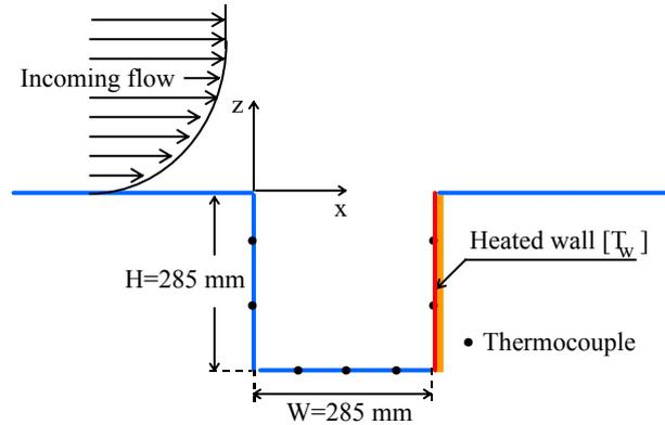
Figure 5: Diagrammatic layout of wind tunnel and canyon model
