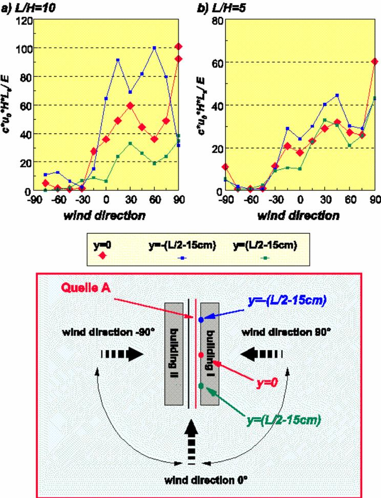
Figure 4: Evolution of the non-dimensional concentration with the wind direction for two different building lengths at  $z=0.0833H$ .
