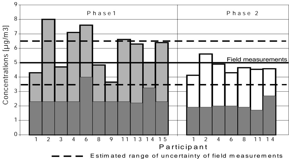
Fig. 3.1.4: Comparison of the calculated annual mean of the total concentration for benzene to each other and to the results of the field measurements. Lower part of columns are the background concentrations taken into account
