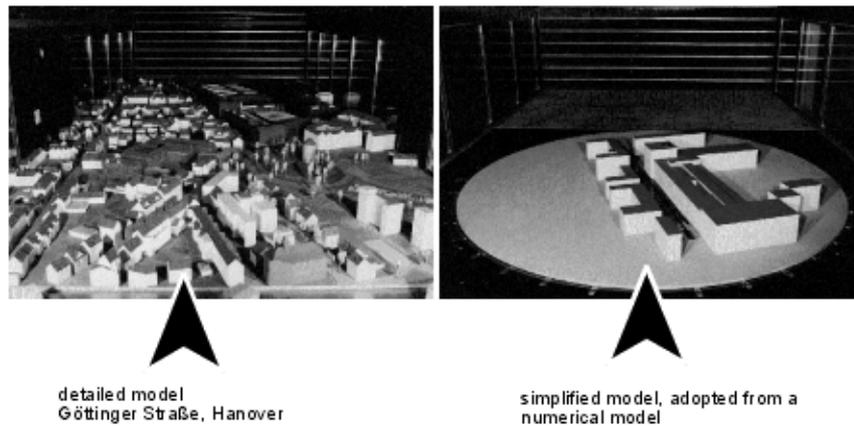
Figure 6: Wind tunnel model for pollutant dispersion investigation
