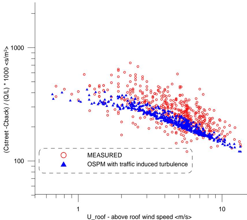
Fig 1.7.1: Measured and calculated additional street  $\text{NO}_x$ -concentrations  $(c_{street} - c_{back}) / (Q/L) * 1000$  in  $\text{s/m}^2$  as a function of the wind speed. Measurements: Wind direction is  $270^\circ \pm 5^\circ$ , plotted are only cases with more than 1000 vehicles per hour and nearly equal distribution of traffic over the 4 lanes. From Clai et al. (2000).
