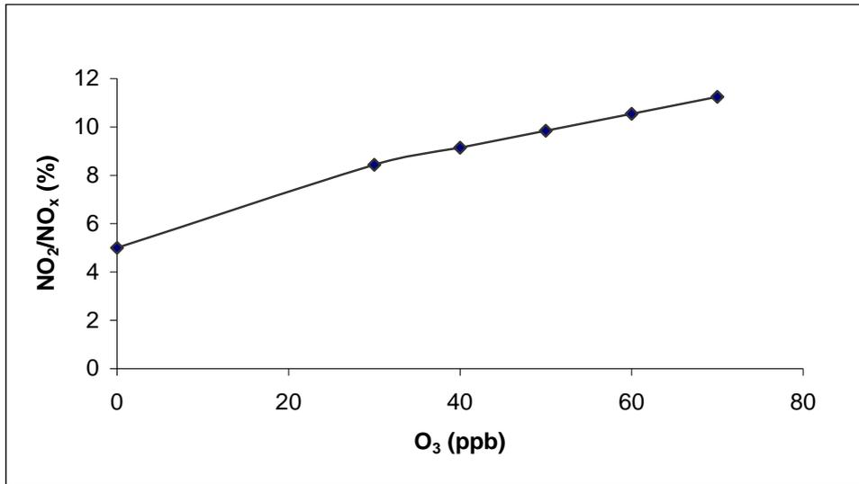
Figure 6: Average NO<sub>2</sub>/NO<sub>x</sub> ratio versus background O<sub>3</sub> concentration as computed by MIMO for the leeward wall.
