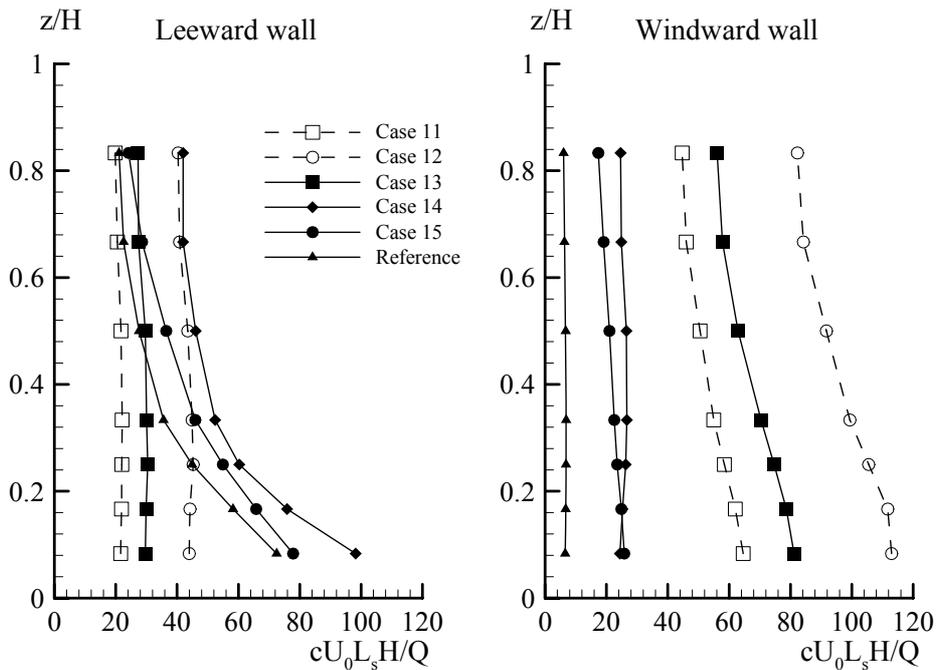
Figure 8: Non-dimensional concentration profiles on leeward and windward walls for different roof shape when considering both leeward and windward roofs
