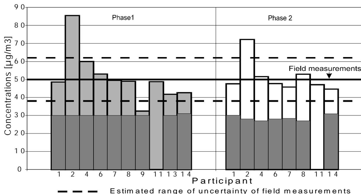
Fig. 3.1.5: Comparison of the calculated annual mean of the total concentration for NO<sub>2</sub> to each other and to the results of the field measurements. Lower part of columns are the background concentrations taken into account. Participant 11 delivered no values for background concentration.
