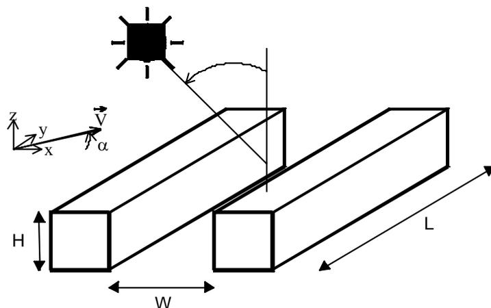
Figure 1: Schematic representation of simple street canyon geometry
