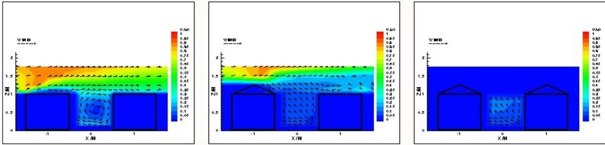
Figure 3: Influence of roof shapes on the flow pattern in an isolated 2D street canyon configuration.
