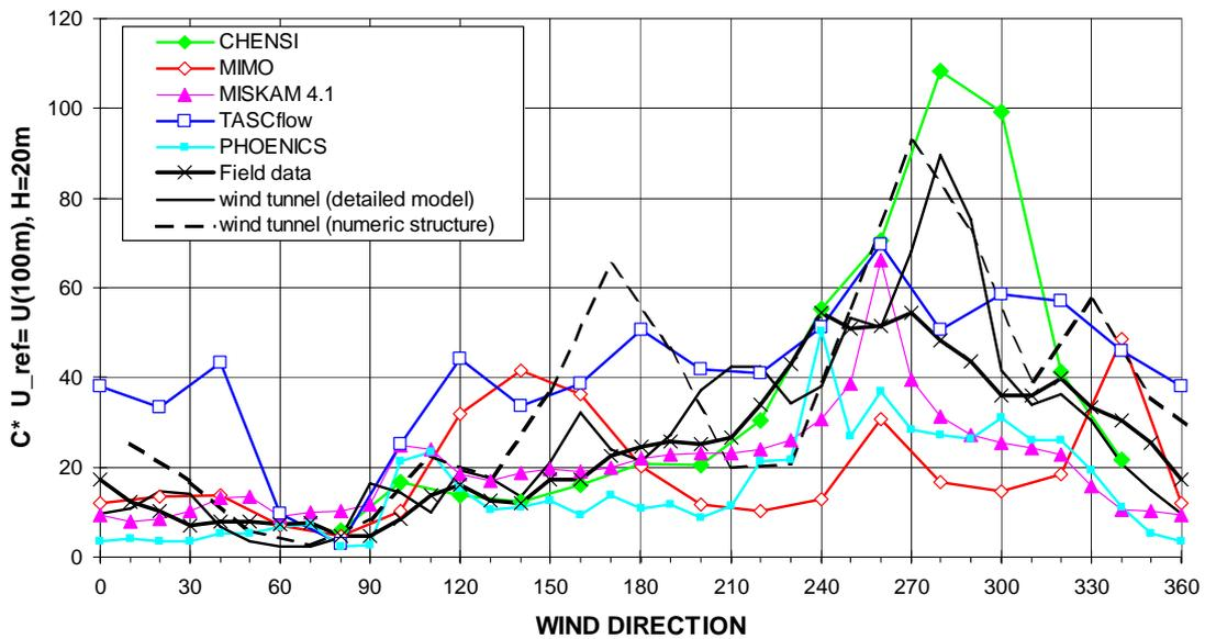
**Figure 2.2.4:** Normalised concentrations versus the wind direction calculated by 5 CFD codes and measured in the full-scale experimental site and in the wind tunnel.
