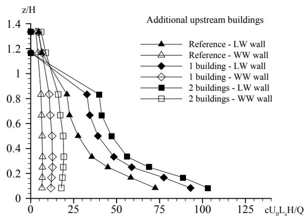
Figure 4: Influence of additional upwind buildings on vertical concentration profiles along the leeward (LW) and windward (WW) walls of a 2D street canyon.
