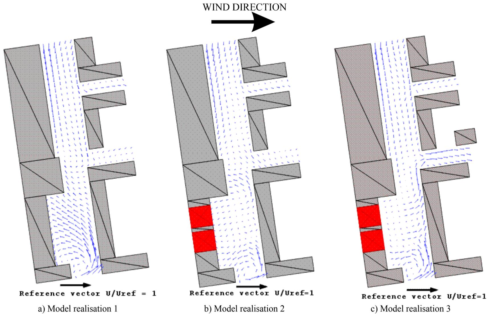
Figure 10: Flow patterns in Goettingerstrasse for three different model realisations and a specific wind direction.
