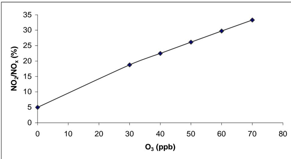
Figure 7: Average NO<sub>2</sub>/NO<sub>x</sub> ratio versus background O<sub>3</sub> concentration as computed by MIMO for the centre of the canyon.
