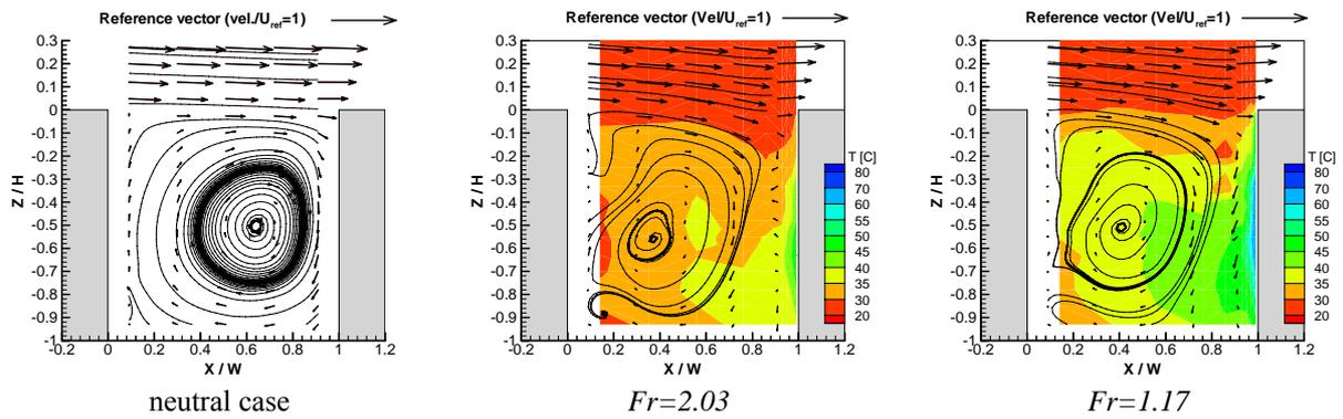
Figure 2: Influence of wall heating on the flow pattern inside a 2D cavity with aspect ratio  $W/H = 1$ .
