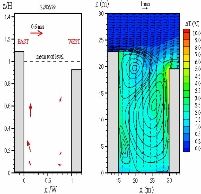
Figure 4: Measured (left) and simulated (right) flow in the street (22/6/99 – 11:00).
