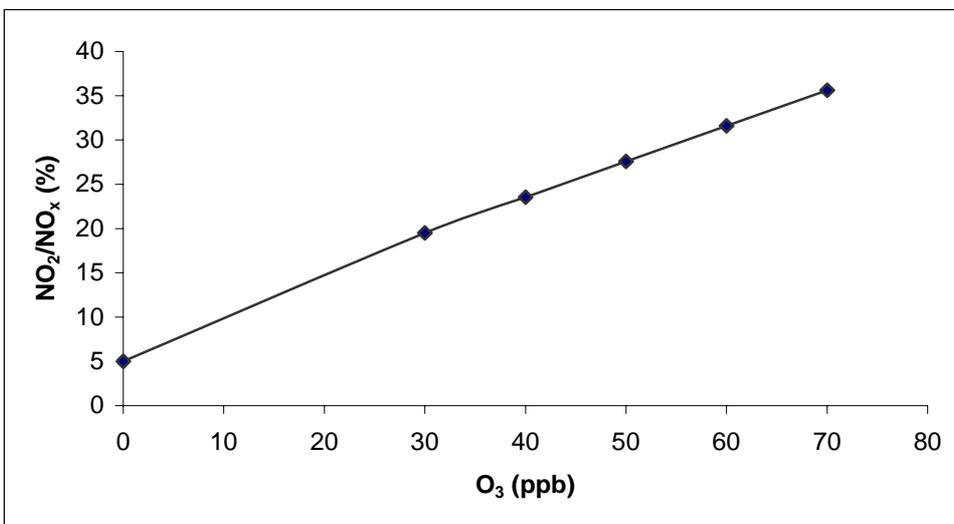
Figure 8: Average NO<sub>2</sub>/NO<sub>x</sub> ratio versus background O<sub>3</sub> concentration as computed by MIMO for the leeward wall.
