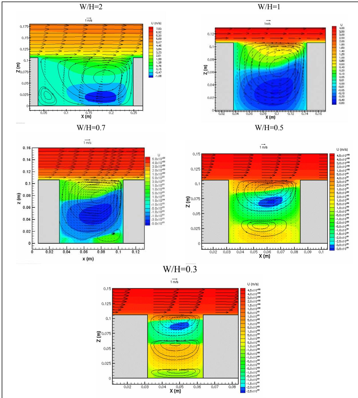
Figure 3a: Variation with aspect ratio (W/H) of flow pattern in a 2-D canyon (CHENSI predictions)
