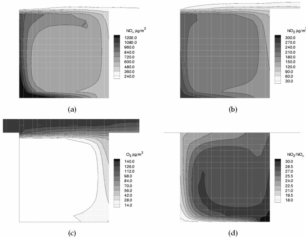
Figure 3: Pollutant concentrations as predicted with CFX-TASCflow. (a) NO<sub>x</sub>, (b) NO<sub>2</sub>, (c) O<sub>3</sub> and (d) NO<sub>2</sub>/NO<sub>x</sub> (%).
