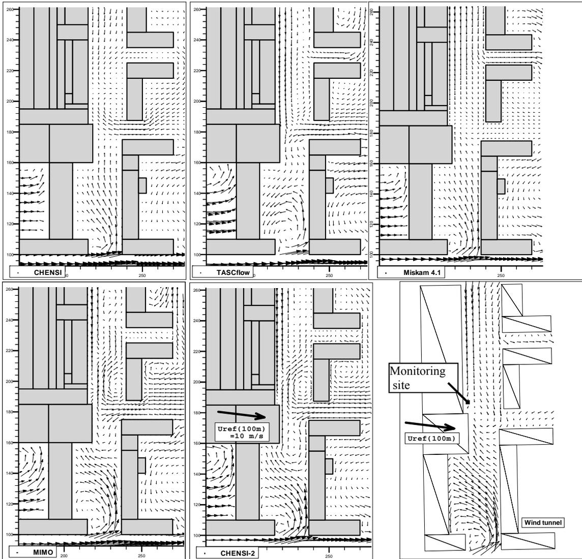
**Figure 2.2.3:** Flow field in horizontal plane calculated by the CFD models and measured in the wind tunnel (wind direction 260° from the North).
