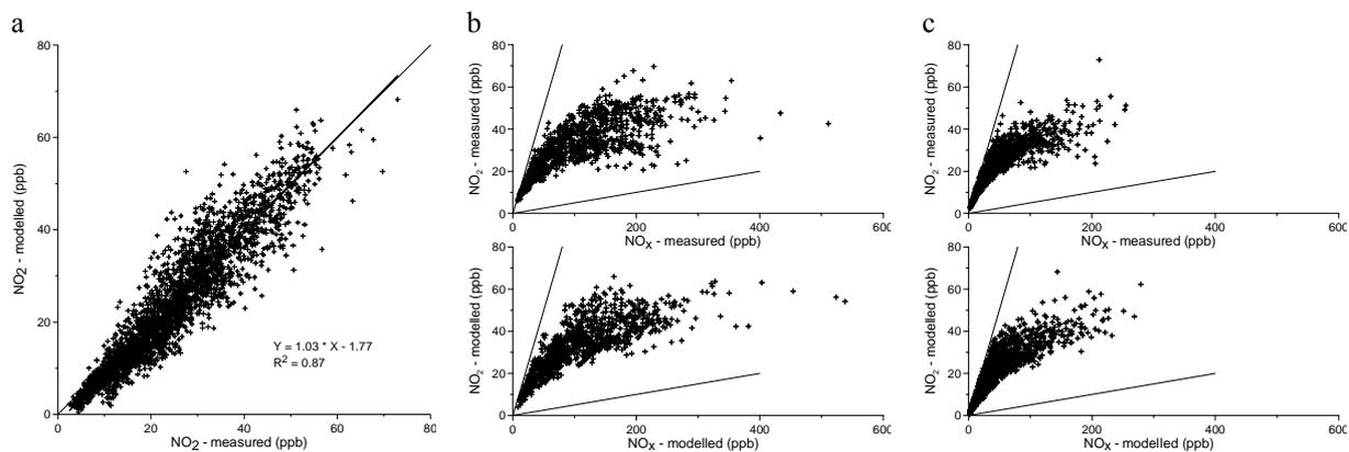
Figure 9. a) Comparison of the measured and modelled NO<sub>2</sub> concentrations for the whole dataset. b) The NO<sub>x</sub> - NO<sub>2</sub> relationships for the leeward side of the street. c) The NO<sub>x</sub> - NO<sub>2</sub> relationships for the windward side of the street. The straight lines shown in b) and c) correspond to the limits of complete oxidation (1:1) and to direct emissions only (0.05:1).
