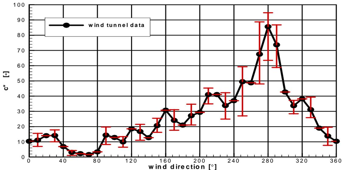
Fig 1.7.2: Variability of short-term averages of measured concentrations. From Liedtke et al. (1998). Measurements in the wind tunnel with averaging times, corresponding to 0.5 hour means in the field.
