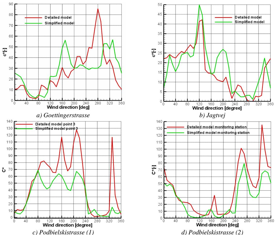
Figure 7: Comparison of dimensionless concentrations as a function of wind direction for detailed and simplified model realizations of three different street canyon configurations.
