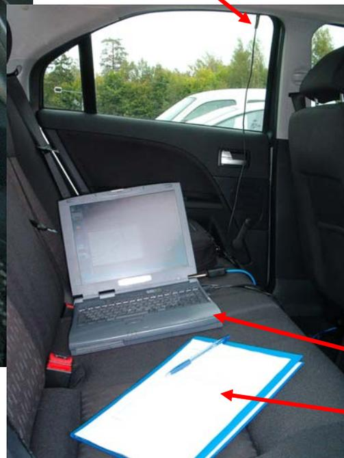
Data logger (time, vehicle speed, rpm, % load, % throttle position)
