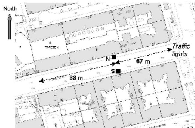
**Figur 5.** Hornsgatan monitoring station North (N) and South (S). The houses are of similar height, 24 m, total street width is 24 m. Uphill slope westward is 2.3% (Gidhagen et al., 2004). Measurements of PM10 are only done on the north side (<http://www.slb.nu/>).
