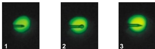
A viewport in the instrument allows you to watch the capillary tip during operation. Three views of the capillary tip are shown above: (1) no liquid flow, (2) with liquid flow but no electrical field, and (3) with liquid flow and an electrical field. The latter view illustrates stable Electrospray operation.
