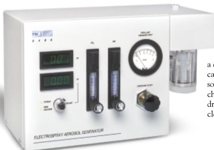
flow transports the droplets to the neutralization chamber. The highly charged droplets are neutralized by a radioactive source (Polonium 210), and the liquid evaporates before the aerosol exits the instrument.
