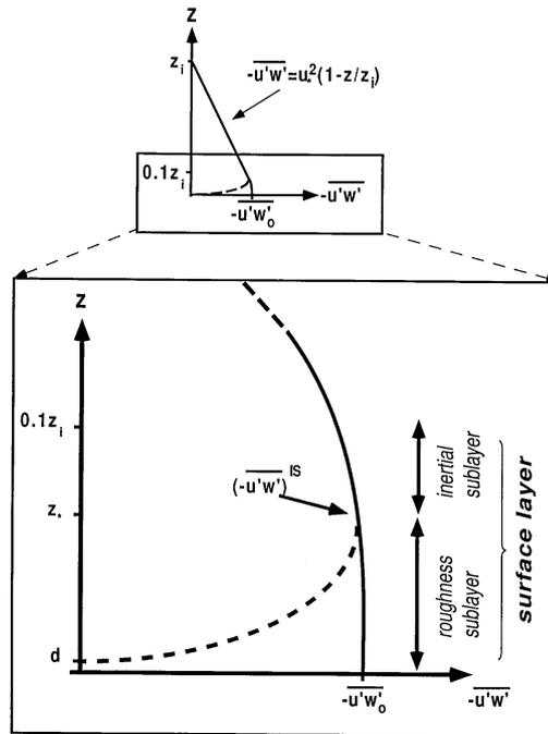
Fig. 8.1: Conceptual sketch of Reynolds stress in the urban boundary layer. The solid line corresponds to a parameterisation according to de Haan and Rotach (1998), which departs slightly from the ‘standard’ linear profile (the upper part of the figure) in that it assumes an approximately constant value when approaching the surface (from Rotach, 2001).  $z_i$  denotes the top of the atmospheric boundary layer.  $u_{*IS}$  referred to in the text equals  $-\overline{u'w'}^{IS}$ .
