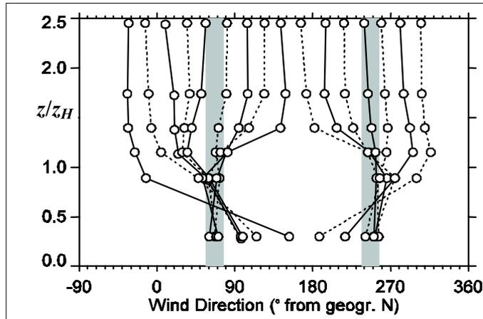
Figure 8.4: Channelling of the flow into the street canyon. Shown is the local horizontal wind direction at the six measurement heights,  $z/z_H$ , as a function of the overlying wind direction sector at the tower top for Sperrstrasse, Basel. The grey bars indicate the street canyon orientations  $67^\circ$  and  $247^\circ$  from geographical north (from Christen *et al.*, 2003).
