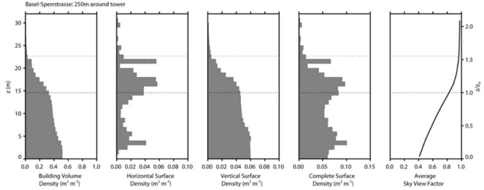
Figure 8.9: Vertical profiles of morphometric properties of the surface in a 250 m circle around the site Sperrstrasse. Data extracted from the digital 1m building model of the city authorities (GVA Basel-Stadt). The dash-dotted line denotes the height of  $u_{* \max}$ . The dotted line denotes the mean height of the buildings.
