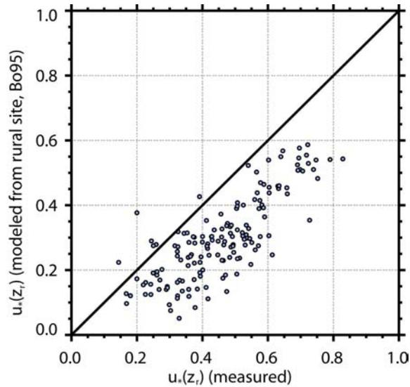
Figure 8.11: Comparison of the measured urban Reynolds stress at  $z^*$  with its modelled values based on the measurements from the rural site Village Neuf and by applying the formula of Bottema (1995), equation (8.4). Shown are hourly averages from May 6 to July 13, 2002, with the wind from Sector B. Under this flow, rural measurements are undisturbed by the city.
