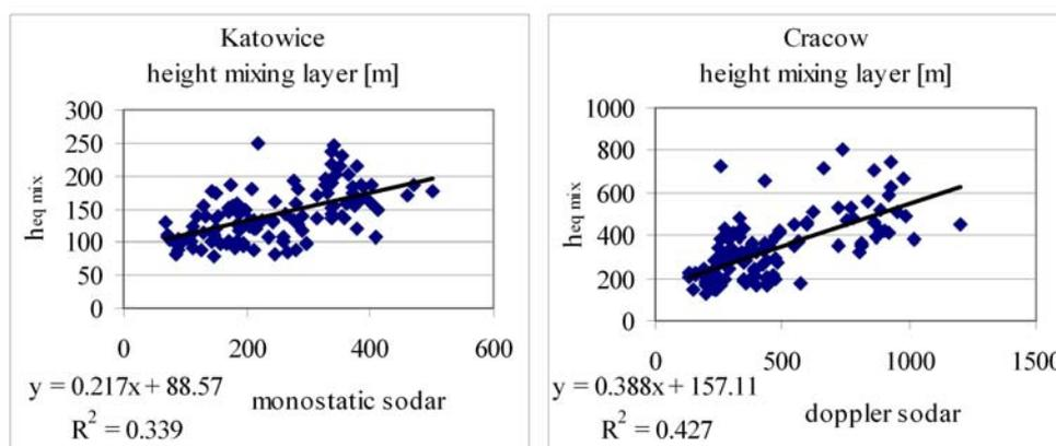
Figure 5.8: Comparison of mixing heights calculated from  $^{218}\text{Po}$  tracer gas concentrations ( $h_{eqmix}$ ) and those observed by a monostatic sodar (Katowice) and Doppler sodar (Cracow).
