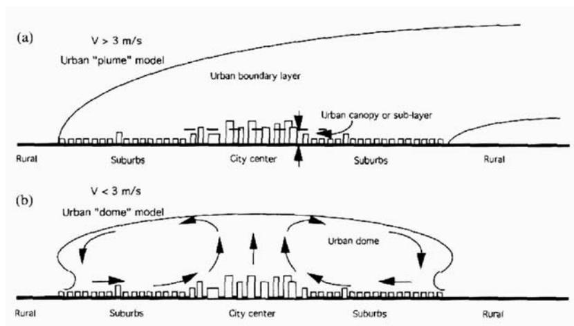
Fig A.3: Schematic representation of the urban heat island in conditions of (a) moderate to strong winds and (b) weak winds
