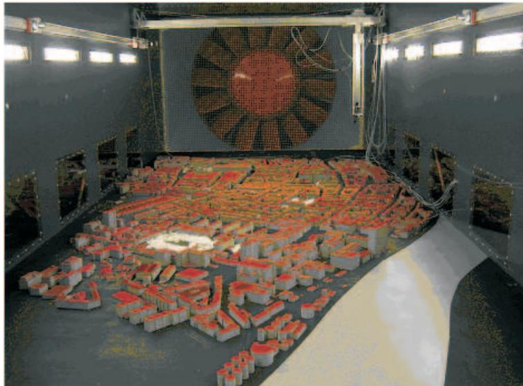
Fig. 10.4 Model of the inner part of the City of Basel in the Hamburg wind tunnel. The white stripe in the foreground corresponds to the River Rhine.
