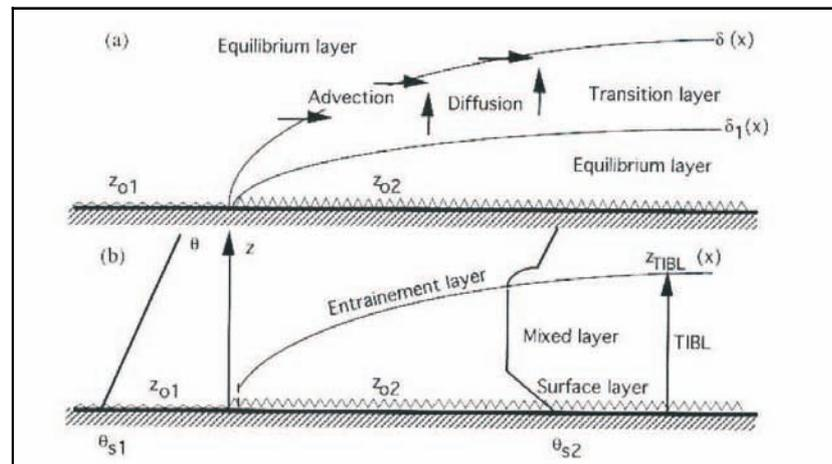
Figure A.2: The development of an internal boundary layer at a transition to a rougher surface: (a) after Hunt and Simpson(1982), (b) after Melas and Kambezidis (1992)
