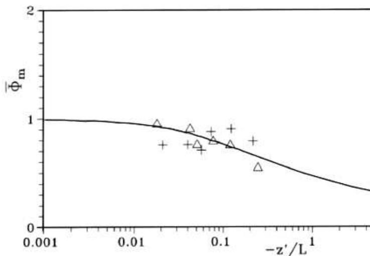
Figure 8.3: Non-dimensional gradient of wind speed averaged over bins of stability under unstable conditions. Data from Zürich, Switzerland (Rotach, 1993b).  $\Delta$  10m above roof level, + 5m above roof level (from Rotach, 1993b).
