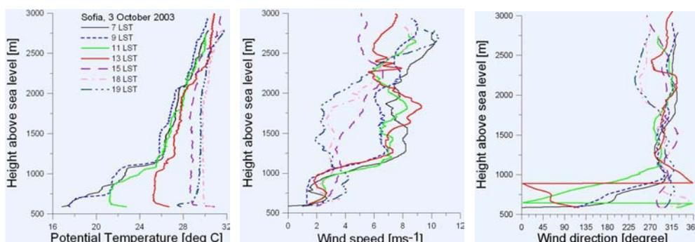
Figure 11.2: Sequence of high-resolution aerological soundings on 3 October 2003. Local summer time (LST) is used. Sunrise is at 7.24 and sunset at 19.06. Potential temperature (left), wind speed (middle) and wind direction (right) profiles are shown.
