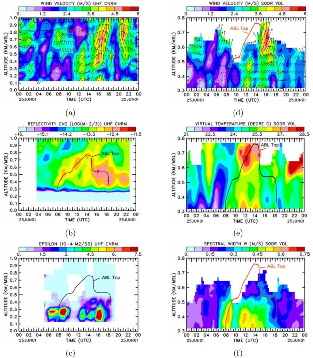
Figure 5.4: Time-height sections of UHF profiler at the Observatoire (left) and sodar-RASS at Vallon Dol (right): (a), (d) Horizontal wind velocity, (b)  $C_n^2$  reflectivity (e) virtual temperature (c) sodar Doppler spectral width, and (f) dissipation rate of turbulent kinetic energy  $\epsilon$ . The superimposed line is the top of the atmospheric boundary layer deduced from the maximum UHF reflectivity.
