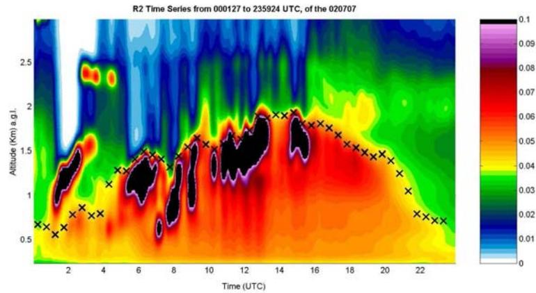
Figure 5.1 Lidar scans of the backscatter from the atmosphere on 7 July 2002 at a site in central Basel, Switzerland. The colour coding is proportional to the aerosol concentration (black=clouds). Crosses indicate the diagnosed aerosol mixed layer height from the derivative of the logarithm of the range-corrected signal. (Data courtesy of Valentin Mitev and Giovanni Martucci, Neuchâtel Observatory.)
