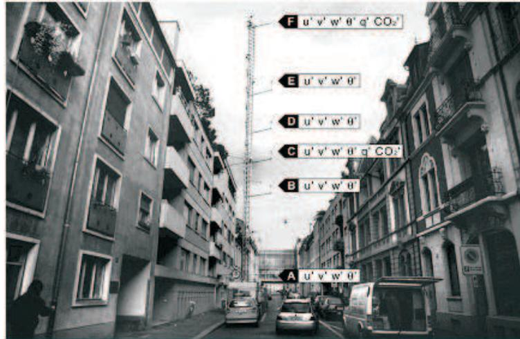
Fig. 10.2: Experimental tower at site Ue1. The arrows indicate the variables measured at the respective levels.
