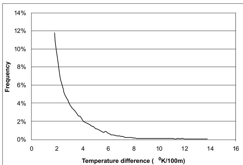
Figure 5.6: The frequency distribution of the potential temperature differences ( $^{\circ}\text{K}/100\text{ m}$ ) for cases with a stable atmospheric stratification, evaluation based on mast measurements at the heights of 26 m and 91 m at the station Kivenlahti located in the Helsinki suburban area, during 1989–1998 (Karppinen *et al.*, 2001).
