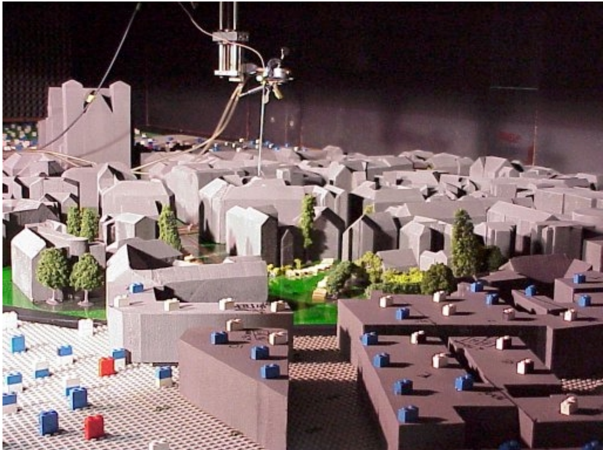
Fig. 4: View of the wind-tunnel model installed at the boundary-layer wind tunnel at the University of Karlsruhe. The situation corresponds to wind direction 243^\circ and the photo was taken upwind the model.
