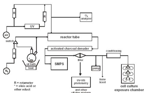
Figure 1. Scheme of the experimental setup.
