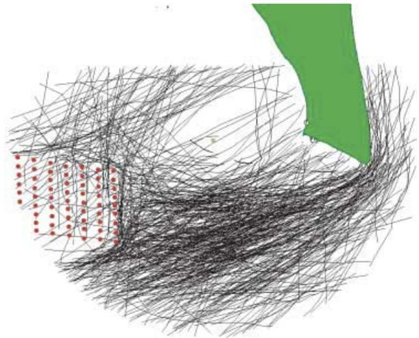
**Figure 2.** Radar registrations from the Nysted offshore wind farm applied on a GIS-platform. Red dots indicate individual wind turbines, green area the land, green dot the siting of the radar, and black lines migrating waterbird flocks determined visually at the Nysted offshore wind farm. Adopted from Kahlert *et al.* 2004.
