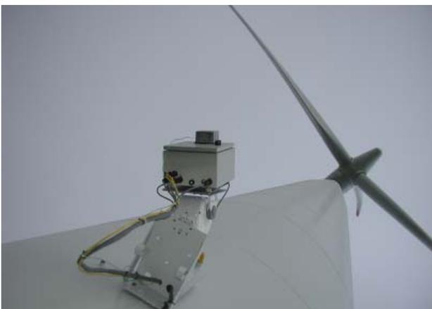
**Figure 10.** The TADS mounted on one of the turbines at the Nysted offshore wind farm. The pan and tilt head is set for vertical collision monitoring. Photo: Mark Desholm/NERI (adopted from Paper II).
