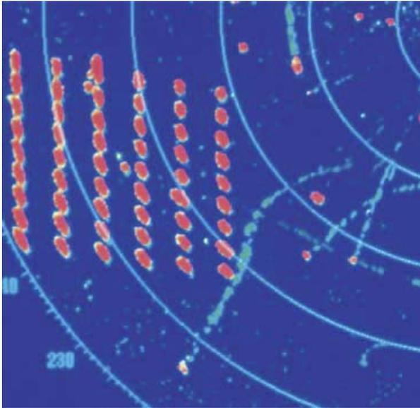
**Figure 1.** Photo showing the echoes of migrating waterbirds (red echoes with green tails) in the vicinity of the wind turbines (red echoes without tails) at the Nysted offshore wind farm, Denmark.
