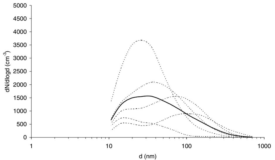
**Figure 3.21.** The full-drawn line shows the average increment of the particle size distribution (cleaned data set). The five broken lines each represent one fifth of the data.
