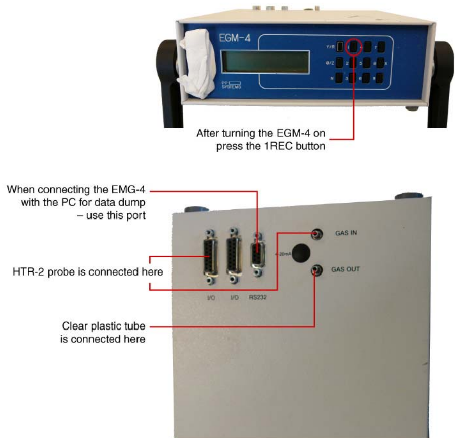
Figure 21. Upper figure shows the EGM4 which is used for measuring CO 2 concentrations. The lower Figure shows the top of the instrument.
