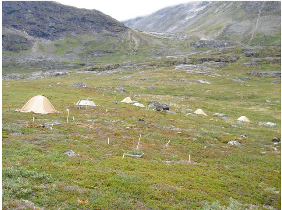
Figure 19. Overview of CO 2 flux plot site with Hessian tents for shading and ITEX hexagons for increasing temperature.
