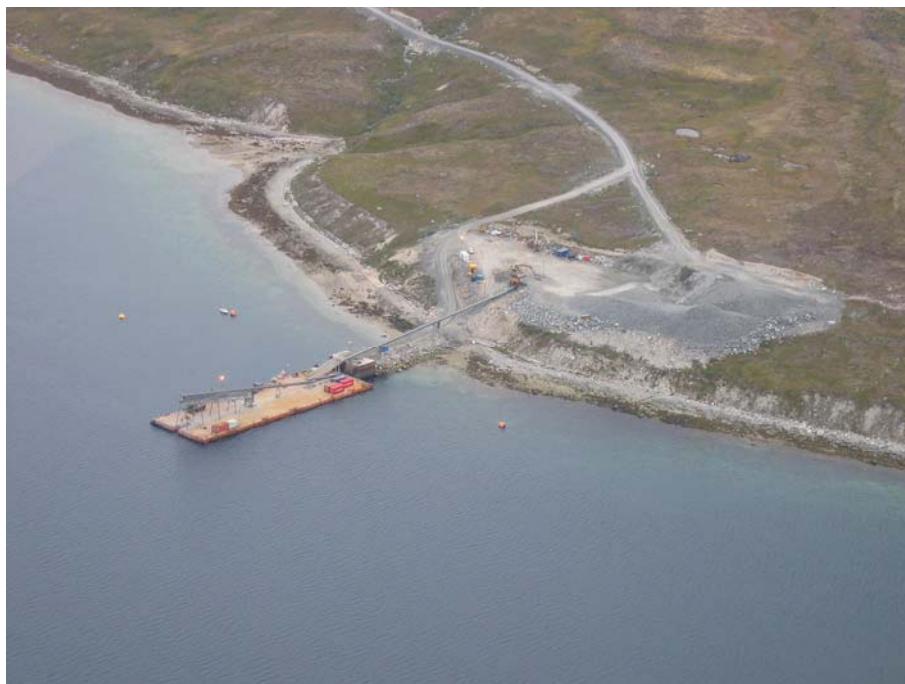
Photo 7. The pier and the barge on the south side of the Kirkespir Bay. In land the stockpile area has a capacity of 60,000 tonnes of crushed ore.
