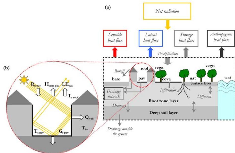
Figure 4.7: (a) Schematic representation of the SM2-U energy and water budget models with 8 surface types (*pav*, *cova*, *bare*, *nat*, *roof*, *vega*, *vegn*, *wat*, see text for explanation) and 3 soil layers, (b) Energy budget of paved surfaces.
