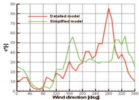
Figure 13.2: Comparison of concentrations measured in the wind tunnel using the detailed and the ‘numerically simplified’ model under otherwise identical conditions
