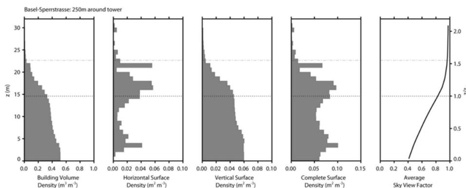
Figure 8.9: Vertical profiles of morphometric properties of the surface in a 250 m circle around the site Sperrstrasse. Data extracted from the digital 1m building model of the city authorities (GVA Basel-Stadt). The dash-dotted line denotes the height of  $u_{* \max}$ . The dotted line denotes the mean height of the buildings.
