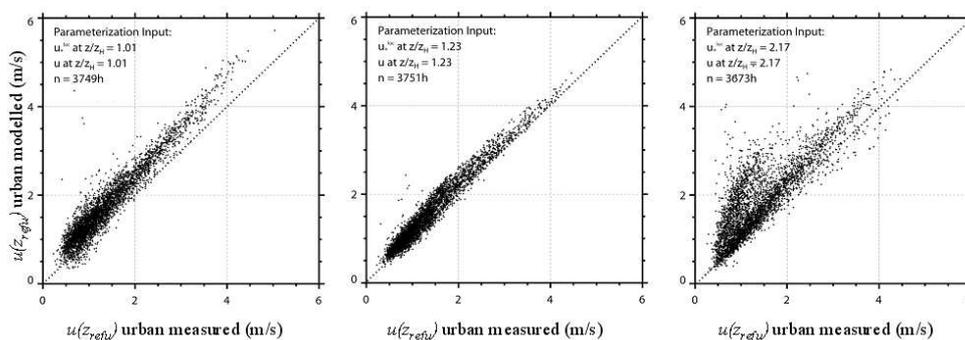
Fig. 3.7: Comparison of measured ( $x$ -axis) and estimated wind speed at an assumed reference level  $z_{ref,u} = d + 10$  m at the site Ue1 (see Fig. 10.1) of the BUBBLE network. The inputs used for the estimation are the mean wind speed and turbulence (1) near roof level (left), (2) near that the reference level (centre) and (3) close to the estimated roughness sublayer height (right). Data are from the BUBBLE project with all stability conditions included (see Chapter 8).
