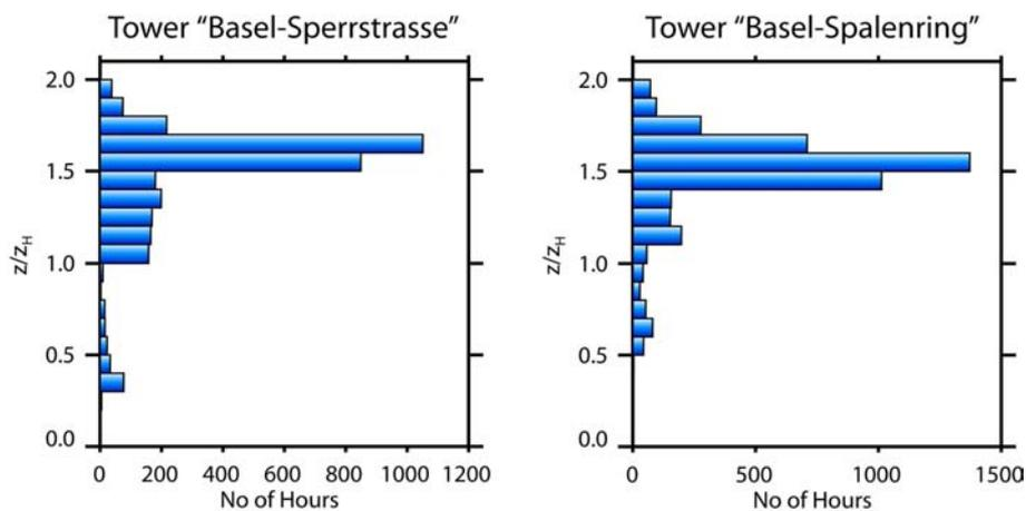
Figure 8.8: The histograms illustrate the height of maximum  $u_*$  at the two urban towers. Data include all stabilities and all wind directions. In the majority of cases, the maximum  $u_*$  is measured close to  $1.55z_H$ . A cubic spline interpolation was performed between measurement levels to enhance the height resolution.
