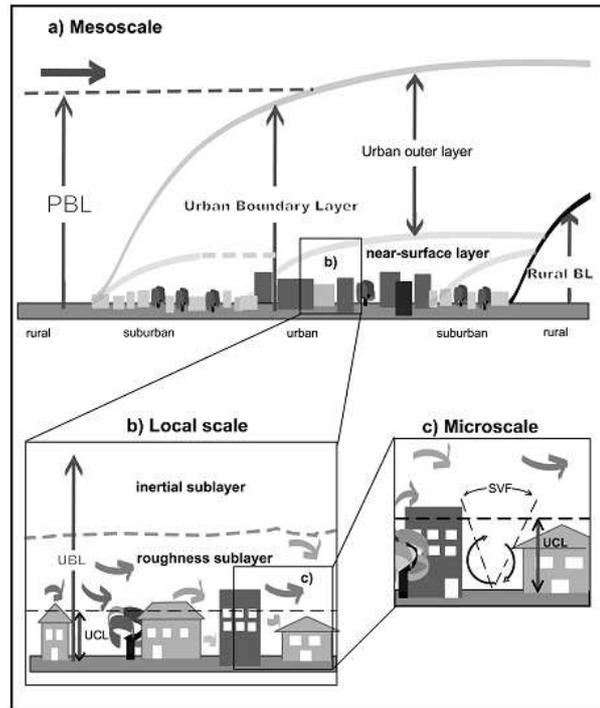
Fig. 2.1: Sketch of the urban boundary layer structure indicating the various (sub)layers and their names (from Rotach *et al.*, 2004, modified after Oke, 1987). An unstable daytime urban boundary layer is shown. For a stable layer of height  $h \cong 200$  m,  $h/z_H \cong 10$  and  $z^*/h \cong 0.1$  to  $0.3$ .
