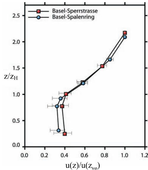
Figure 8.5: Ensemble wind profiles normalised by wind speed at the tower top,  $u(z)/u(z_{top})$ , as a function of height  $z/z_H$  derived from the sonic anemometers for the whole operation period. Error bars indicate the 20% and 75% percentile of all data (Christen *et al.*, 2003).
