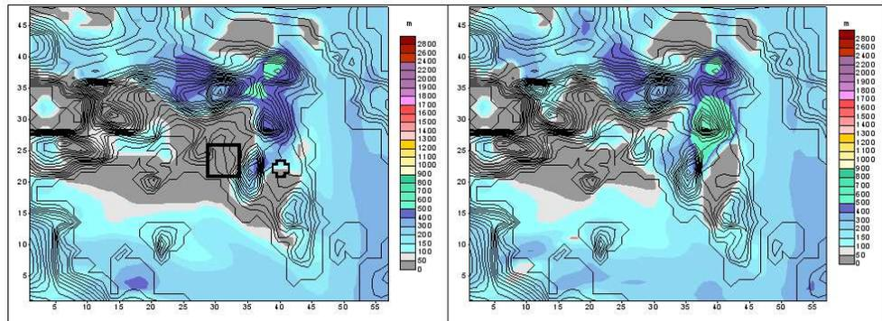
Figure 5.3: Spatial distribution of the mixing height calculated by the original (left) and modified (right) MM5/MRF model, at 23:00 LST on 14 September 1994. The axes represent number of grid cells of 2 km each. Central Athens is indicated by a box in the middle of the left figure, the rural Spata station is indicated by a cross. The urban National Observatory of Athens station is inside the box.
