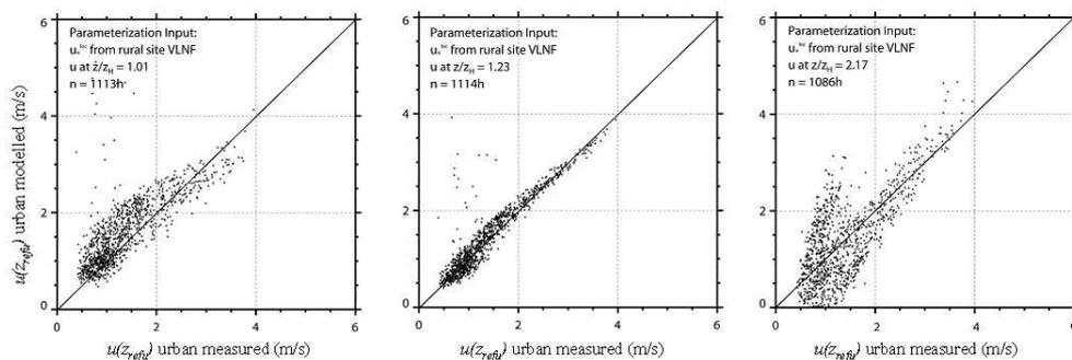
Fig. 3.9: As Fig. 3.7 but only measured ‘rural’ wind speeds are used as input to derive the estimated (‘modelled’ in the label) urban wind speed. The text in the caption ‘ $u_*^{loc}$  from rural site’ is meant to indicate that this value is estimated from mean variables observed at the rural site Village Neuf.
