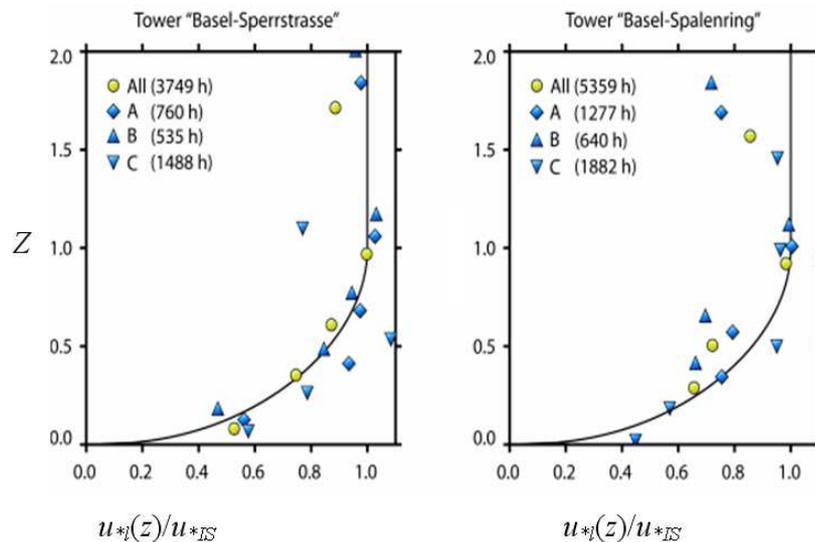
Figure 8.10: Parameterisation of the  $u_*$  profile (black line, equation 8.3) as a function of height  $Z = (z-d)/(z^*-d)$  in comparison with measured values of  $u_{*l}(z)/u_{*IS}$  for all data and for the different wind direction classes A, B and C separately. Observational data are processed with an individual  $h$  for each of the wind sectors,  $d = 0.7z_H$  and  $z^* = 1.55z_H$ .
