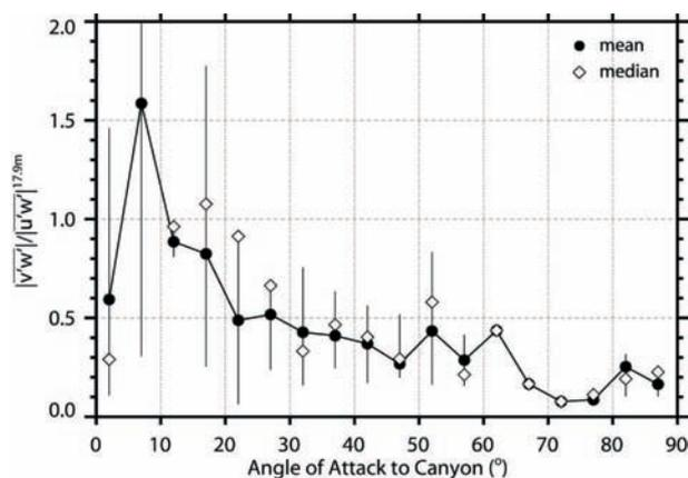
Figure 8.7: The ratio  $\overline{v'w'}$  to  $\overline{u'w'}$  shows the relative importance of lateral contribution to the importance of longitudinal contributions to the vertical flux of momentum at Sperrstrasse. The plot shows the ratio as function of the flow direction relative to the street canyon directly above roof top ( $z/z_H = 1.23$ ) at a height of 17.9m.
