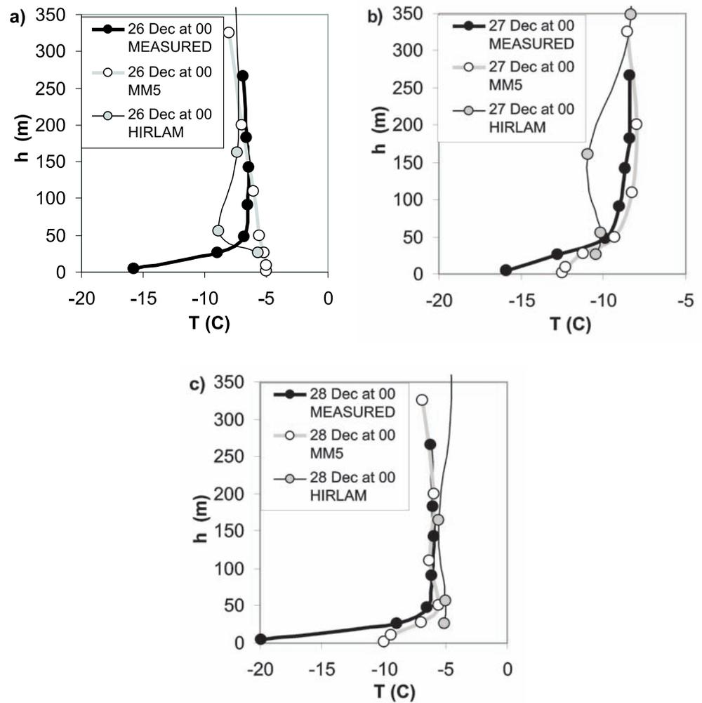
Figures 6.1. a-c: The nocturnal temperature profiles measured at the radio tower of Kivenlahti, and those predicted by the MM5 and HIRLAM models, at 24 hour intervals during 26 to 28 December 1995 (Pohjola et al., 2004). Note the different temperature scale in Fig. 6.1b. Reprinted with permission from Boreal Environment Research.  $h$  denotes height above ground and  $T$  temperature
