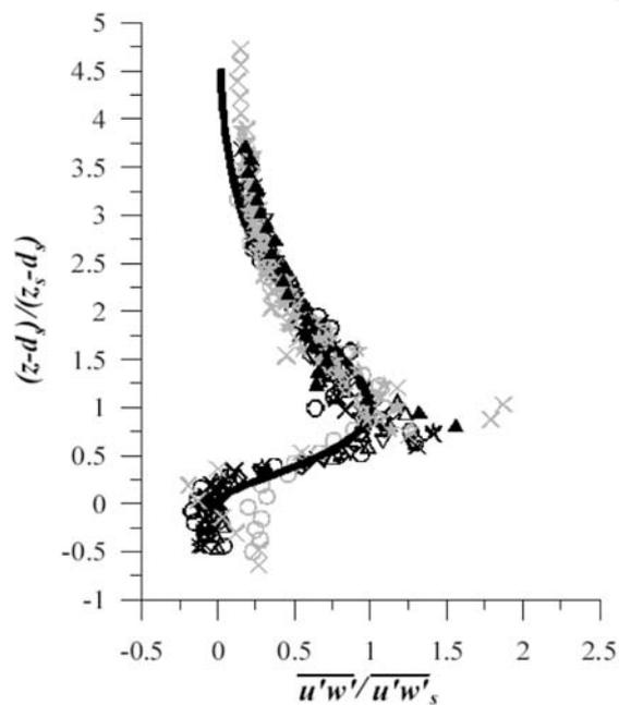
Fig. 3.1: Profiles of suitably scaled momentum flux at 11 different urban sites. Data from a wind tunnel study using a model of the city of Nantes (Kastner-Klein and Rotach, 2004).
