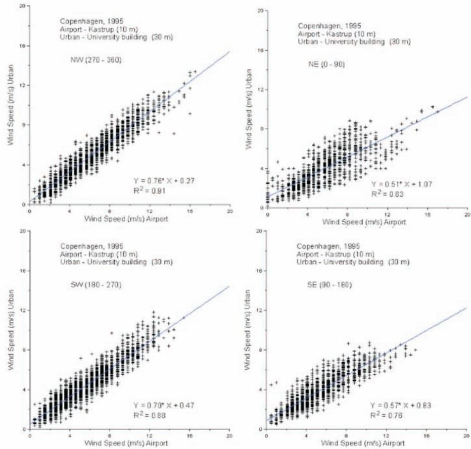
Fig. 3.6: Comparison of hourly wind speeds from the University building station (y-axis) in Copenhagen, Denmark and the nearby Kastrup Airport station (x-axis), according to wind sector. Top left: 270 to 360 degree wind direction; top-right: 0 to 90 degree wind direction; bottom-left: 180 to 270 degree wind direction and bottom-right: 90 to 180 degree wind direction. From Soriano *et al.* (2002).
