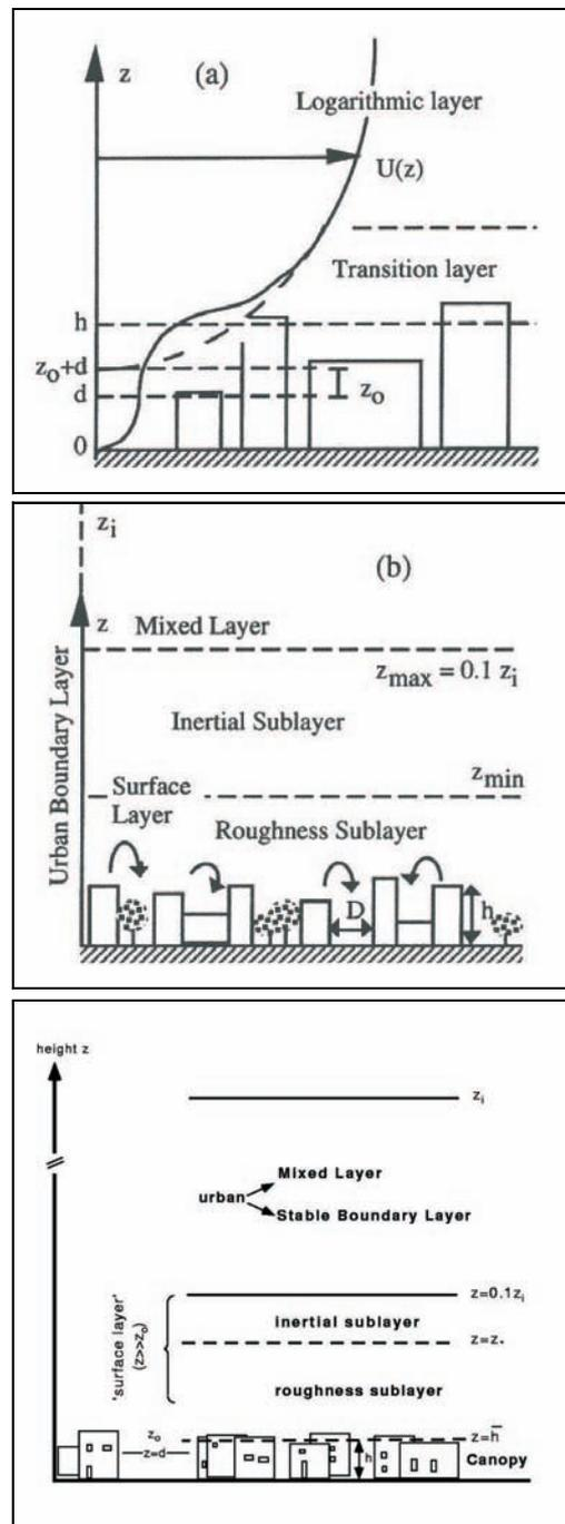
Fig A.1: Schematic representations of the urban boundary layer: (a) after Karlsson (1986), Fochter (1989); (b) after Oke (1988), Rotach (1991), (c) after Rotach(1999)
