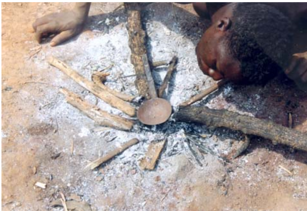
Fig. 3 The gold-mercury amalgam is heated over the fire. The mercury evaporates and the gold is left in the iron cup.
