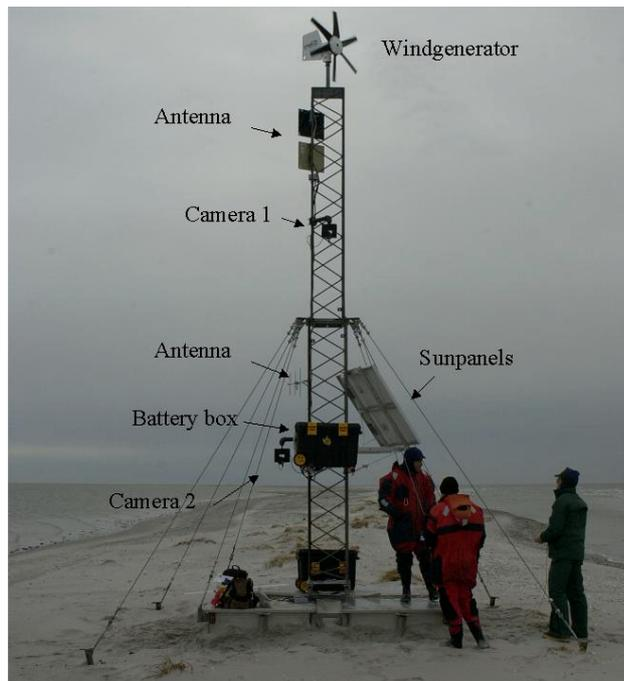
Figure 3.3 Camera tower at Rødsand Seal Sanctuary with antenna, wind generator, solar panels and battery box.
