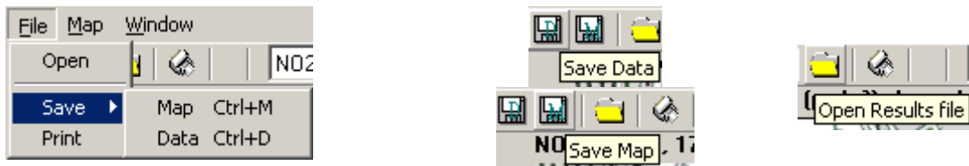
Fig. 14.13. The Multi Streets calculation results can be saved either as a map picture or as a file with numerical data. The corresponding menu items are shown at the left, while the associated icon buttons at the right. To open a previously saved result file you can use the File/Open menu item or the associated icon button.
