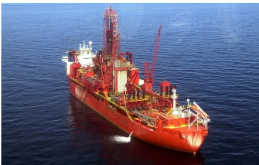
Figure 2.1. The 121,000 tons and 253 m long drill ship West Navion that operated at Qulleq-1 during summer 2000.
