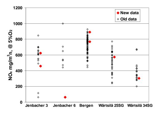
Figure 5  $NO_x$  emission data for natural gas engine makes
