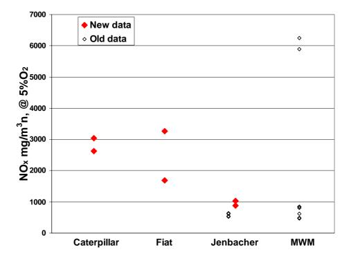
*Figure 13* NO<sub>x</sub> emission data for biogas engine makes
