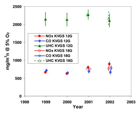
Figure 8 Emission time series for two Bergen natural gas engines
