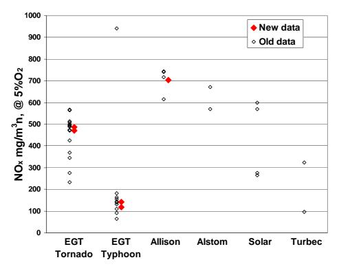
Figure 3 New and old  $NO_x$  emission data for natural gas turbines
