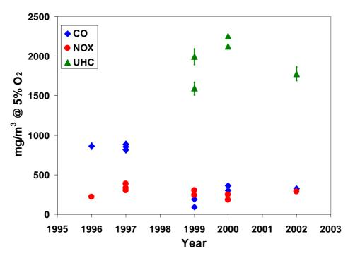
Figure 9 Emission time series for a Caterpillar 3600 natural gas engine. CO catalyst was installed in 1998
