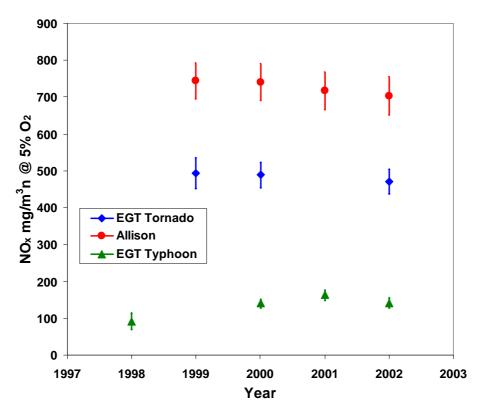
Figure 4 Time series of NO<sub>x</sub> emission data for natural gas turbines. Vertical lines show the uncertainty of the NO<sub>x</sub> measurements.
