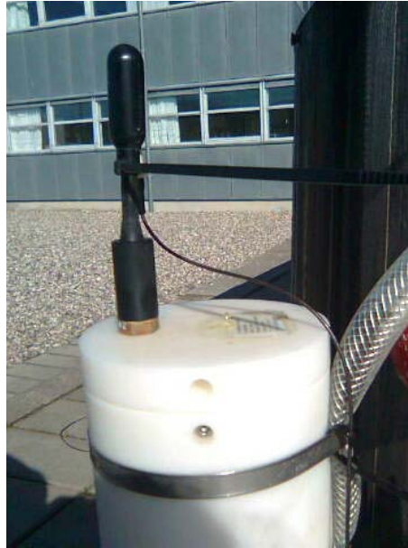
Figure 2.9. DSG-recorder from Loggerhead Instruments. Measuring about 50 cm in height. The black rubber extension is the hydrophone.
