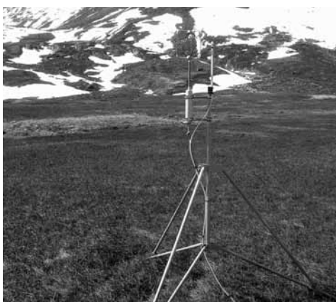
Figure 3.8 The new CO 2 eddy covariance mast was installed in the fen site close to the automatic chambers on 10 June 2008.
