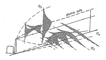
Figure 3 The gaussian plume concept.
