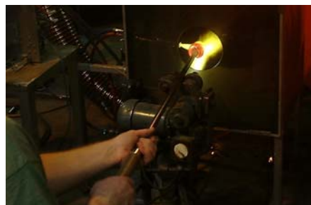
Figure 1. a) A schematic of applying Liquid Flame Spray process for nanoparticle deposition on surface, b) in-situ photograph of a glass colouring session in studio.
