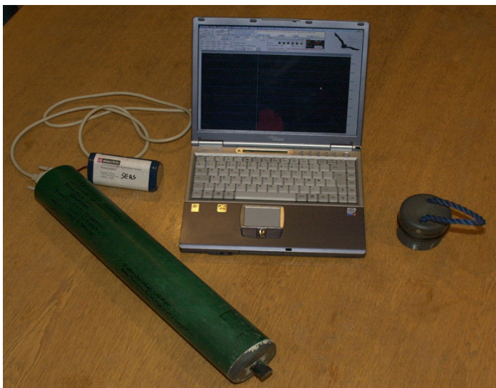
Figure 3. Example of SAM datalogger; a T-POD connected to a laptop for download (courtesy of Jakob Tougaard).
