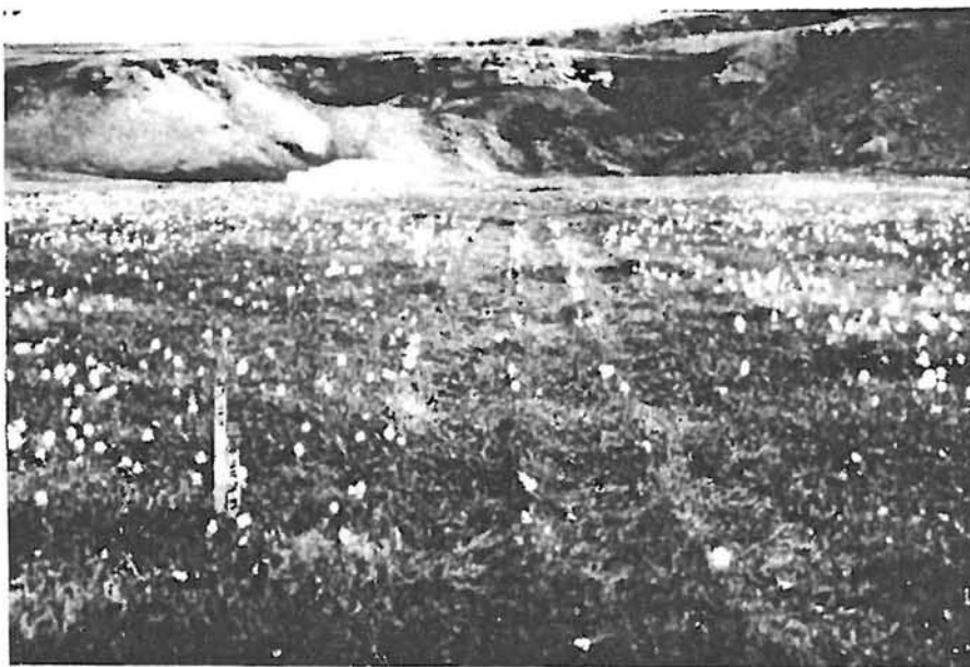
Track from ten passes on sloping terrain is seen. The two outermost depressions is from the rear wheels, and the depression seen in the middle is from the front wheel of the ATC. August 15, 1983.
