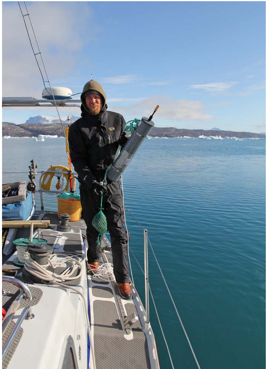
Figure 16. The noise recording equipment, with the hydrophone protruding from the top
