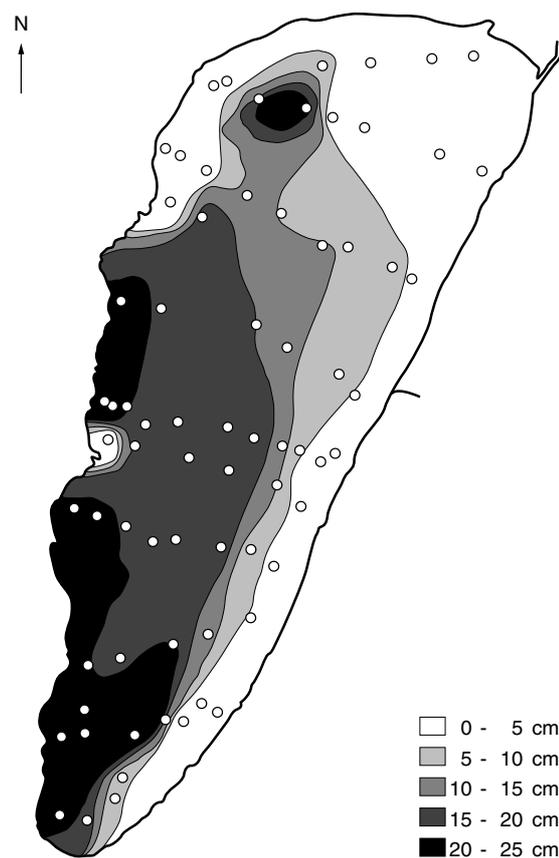
**Figure 2.2** Sediment hardness in Lake Ferring measured as the penetration depth of a metal spear using a penetrometer. Measurement stations are indicated by circles. From Søndergaard *et al.* (2000).
