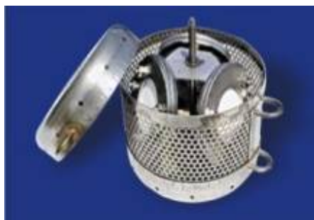
Figur 2.1 POCIS (Polar Organic Chemical Integrative Sampler). Tre passive opsamlere monteret i en rustfri stålurv (Exposemeter).
