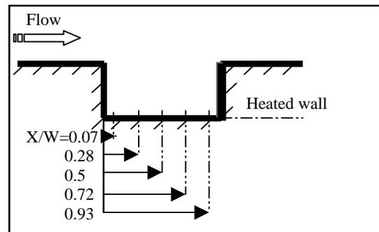
Fig. 2 Description of the measured profiles within the cavity.
