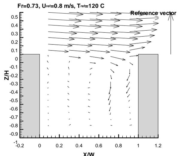
**Fig. 5** Velocity vectors inside cavity, Fr=0.73.
