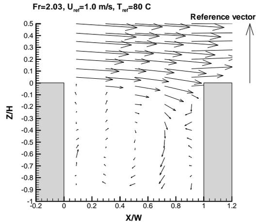
Fig. 7 Velocity vectors inside cavity, Fr=2.03.
