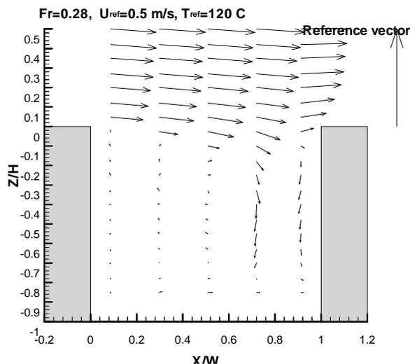
**Fig. 4** Velocity vectors inside cavity, Fr=0.28.
