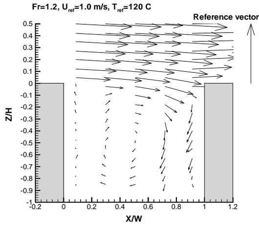
Fig. 6 Velocity vectors inside cavity, Fr=1.20.
