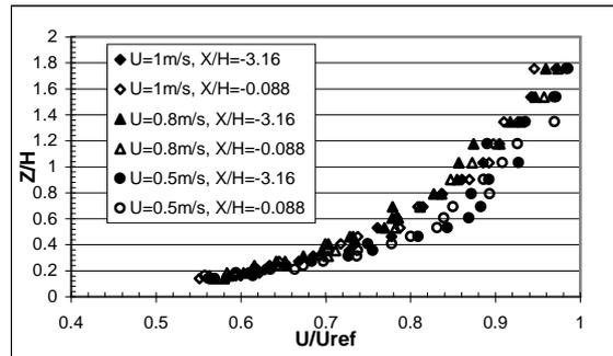
**Fig. 3** The oncoming mean velocity profiles, taken at 3 different velocities and 2 different upstream positions.
