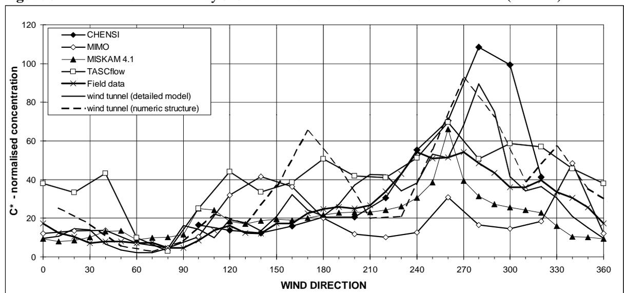
**Figure 4:** Normalised concentrations in the dependence on the wind direction. Calculated by 4 CFD codes, measured in the field and in the wind tunnel.
