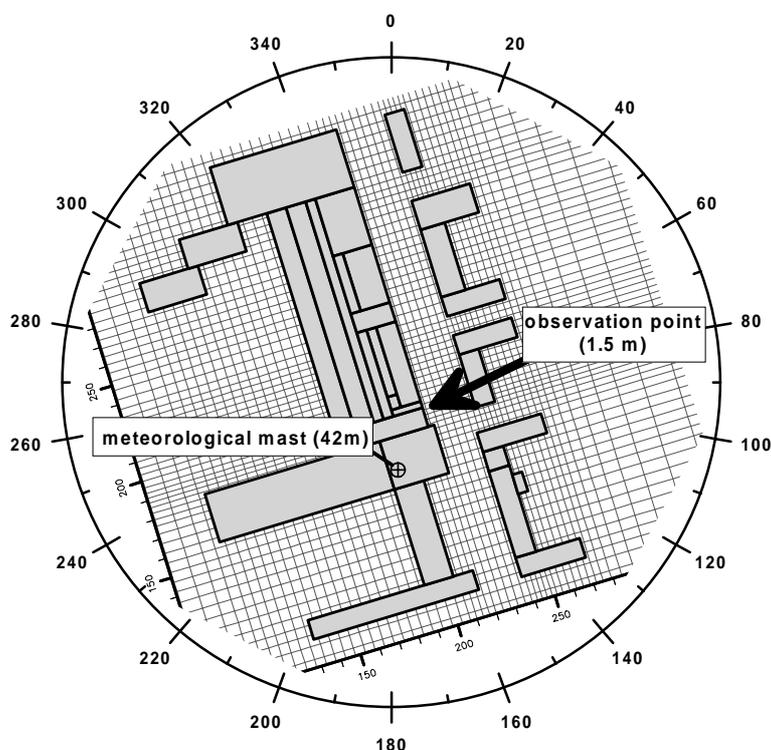
**Figure 2:** Top view on the modelling area. The grey areas indicate buildings. The mesh shows the resolution of the grid. The circular axis gives the direction with respect to North as it is used for the approaching flow direction in Fig.3 and 4.
