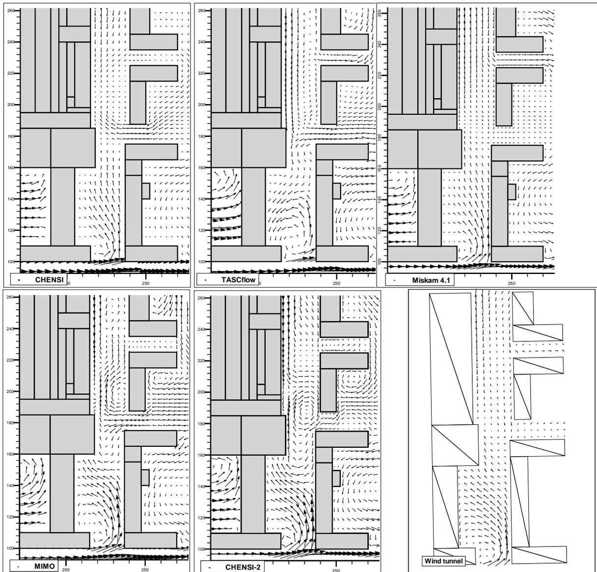
**Figure 3:** Flow fields calculated by 5 CFD codes and measured in the wind tunnel (see text).
