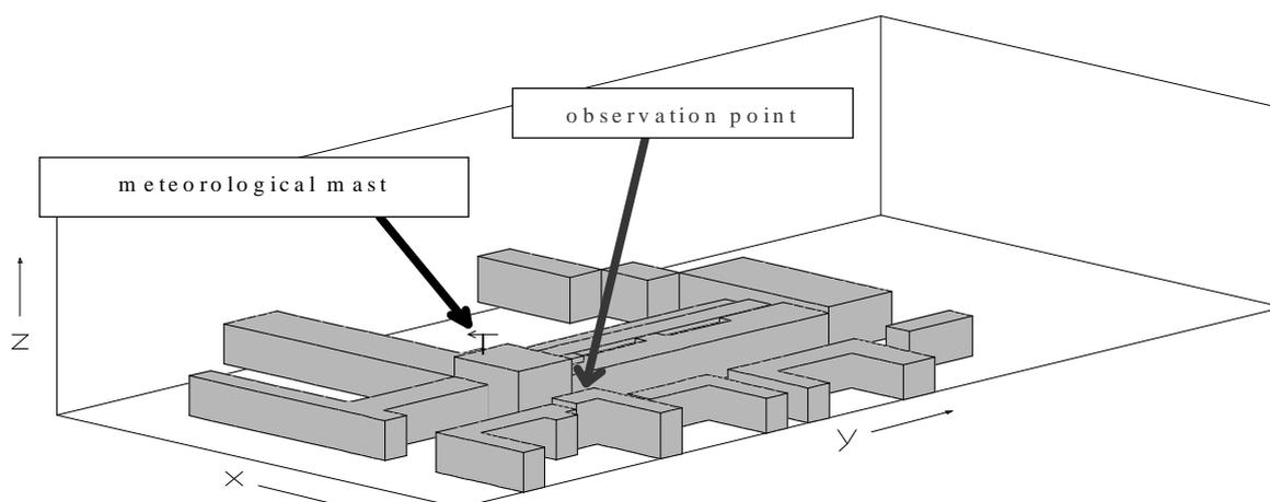
**Figure 1:** Central part of the modelling domain. The position of the meteorological mast and the point of the concentration measurements are indicated in the sketch.
