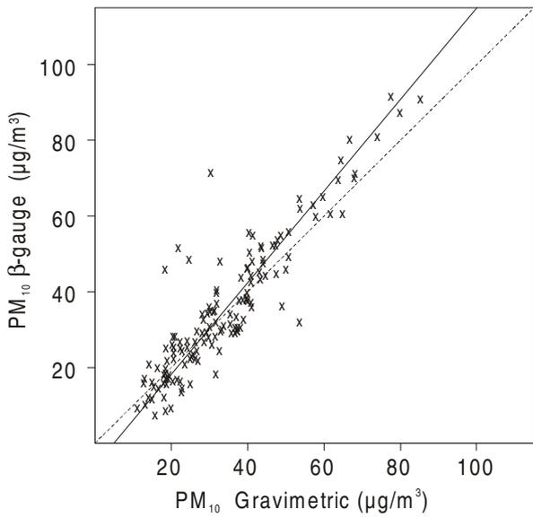
Figure 5.5 Comparison between  $\beta$ -gauge and gravimetric determination of the PM<sub>10</sub> concentration. The dotted line is 1:1 and the drawn line is the orthogonal regression line:  $y = 1.21 x - 5.9 \mu\text{g}/\text{m}^3$  ( $\rho=0.93$ ).
