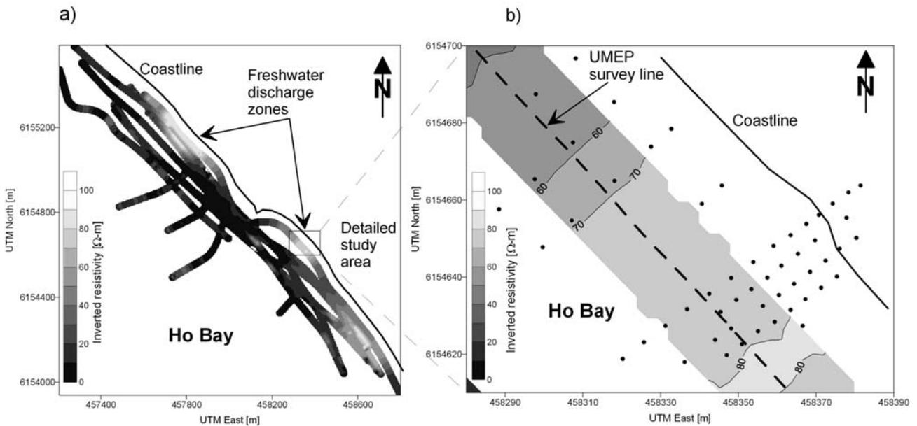
Figure 5. a) UMEP survey lines showing the contoured calculated resistivity ( $\Omega$ -m) of the second layer of the inverted UMEP data. b) Detailed study area showing contoured calculated resistivity ( $\Omega$ -m) of one UMEP survey line. Dots are locations for sampling of sediment pore water.
