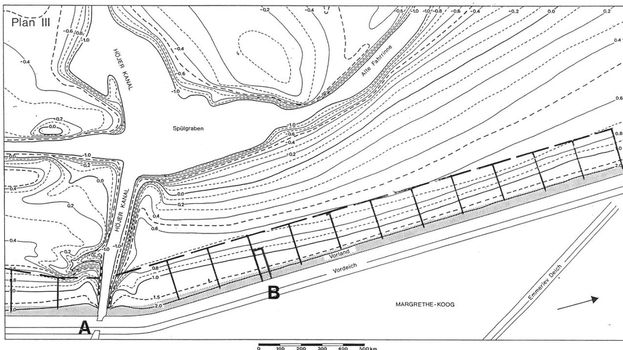
Figure 3. Contour map of the tidal flat and foreland north of the Vidå Sluice 1983/1984, with the sedimentation fields, established in 1988, inserted. A: The Vidå Sluice. B: Permanent study area used in the present study. After Jespersen & Rasmussen 1989.
