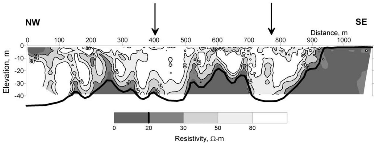
Figure 4. MEP profile along the beach of the study site showing the distribution of freshwater (30-500  $\Omega$ -m). Black line is an interpretation of the aquifer bottom and the arrows indicate the major zones of groundwater discharge.
