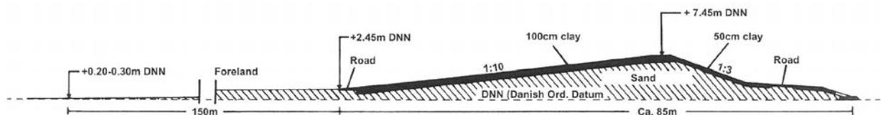
Figure 2. Schematic cross-section of the advanced seawall with the planned, 150 m broad foreland. After Jespersen & Rasmussen (1984).
