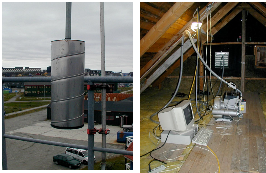
Figure 2.3 Left picture: The inlet to the high volume sampler at the roof of ASIAQ, Nuuk and right picture the pump and the sample flow detection system
