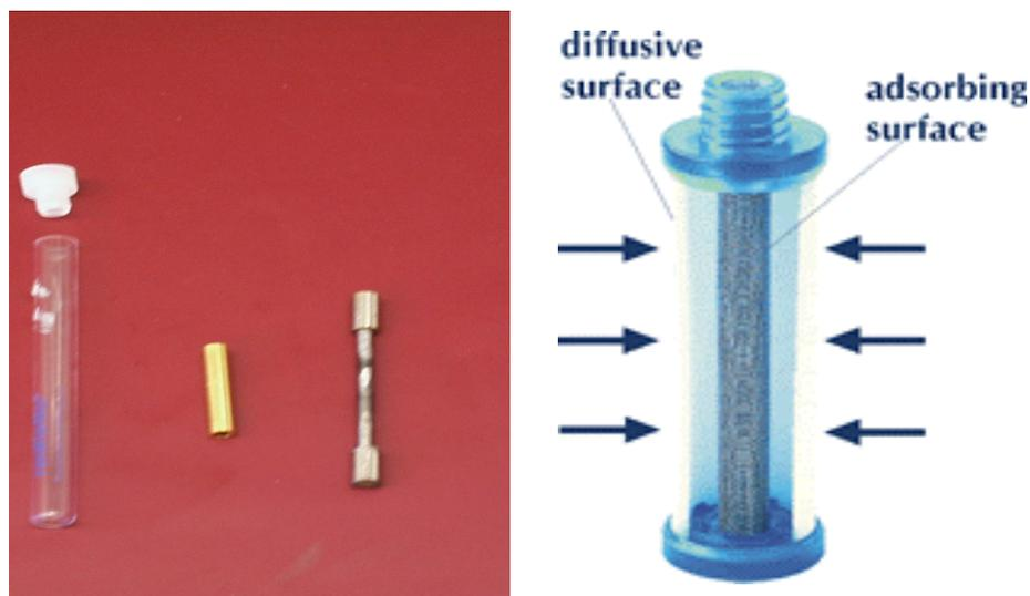
Figure 4.3 Left; Gold core that adsorbs mercury, supporting iron core and glass tube with plastic cap to store the gold core before and after sampling. Right; Radiello diffusive body in polyethylene.
