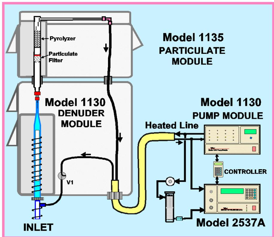
Figure 3.2 TEKRAN fractionation system consisting TEKRAN 2537A cold vapor atomic fluorescence mercury analyzer, equipped with TEKRAN 1130 RGM sampler and 1135 FPM sampler. From [www.tekran.com](http://www.tekran.com).
