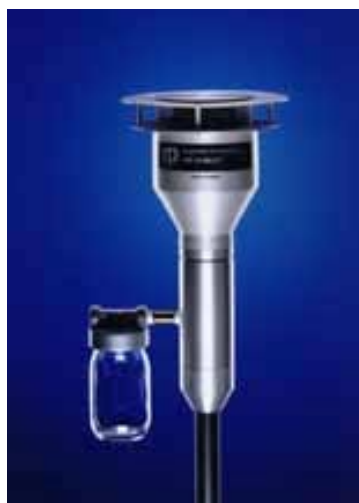
Figure 8 PM_{10} is measured by collection of particles on a filter. The inlet (shown left) cuts off particles > 10 \mu\text{m} . The graph (shown right) shows that the cutoff is not sharp, but defined by the reference method.
