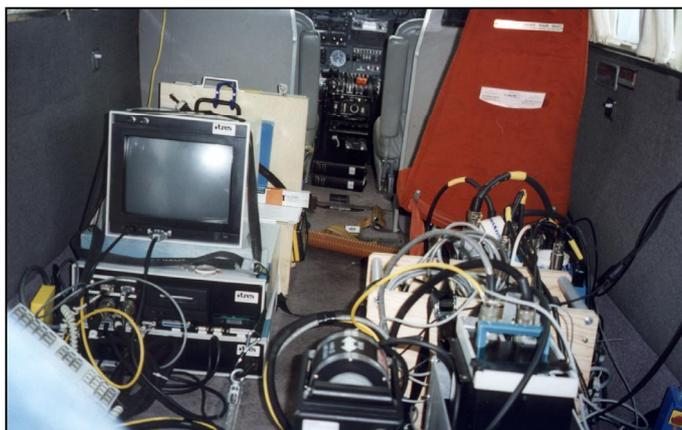
Figure 14: The *casi* scanner as installed in the aircraft for image acquisition. Photo: M. Stjernholm.
