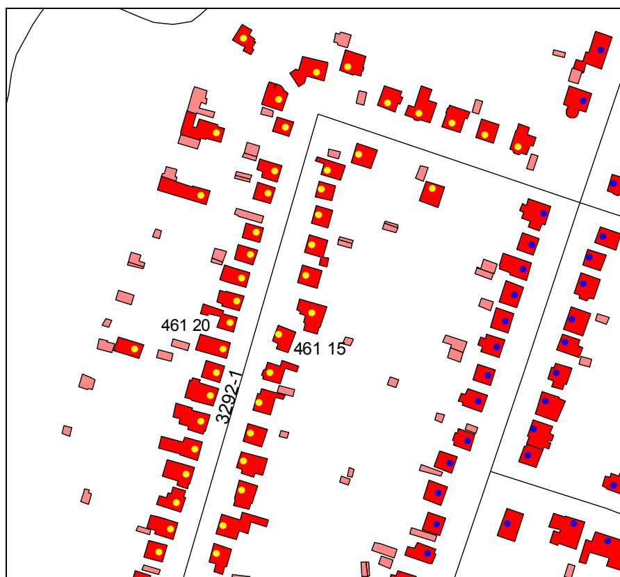
Figure 4.19 Example of missing match between the road codes of the address and the adjacent road. The addresses along a road have the road code 461 but the road is defined by the road code 3292.
