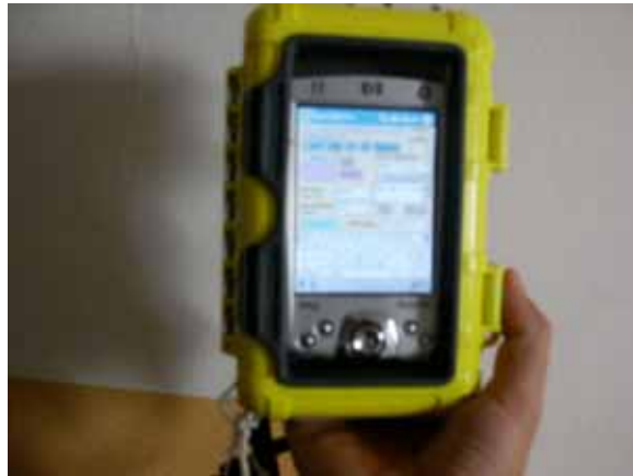
Fig.1: PDA in waterproof case used while Mesohabitat mapping for MesoCASiMiR
