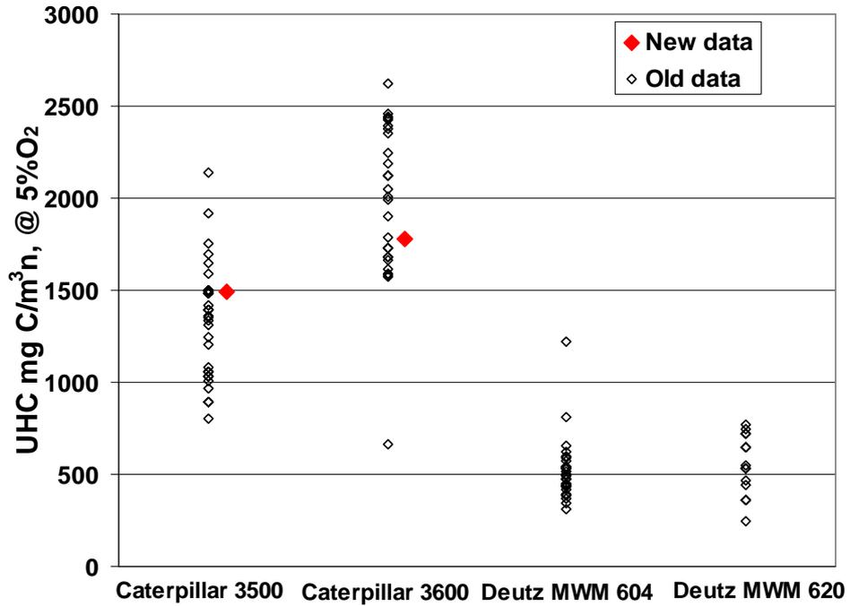
Figure 7 UHC emission data for natural gas engine makes
