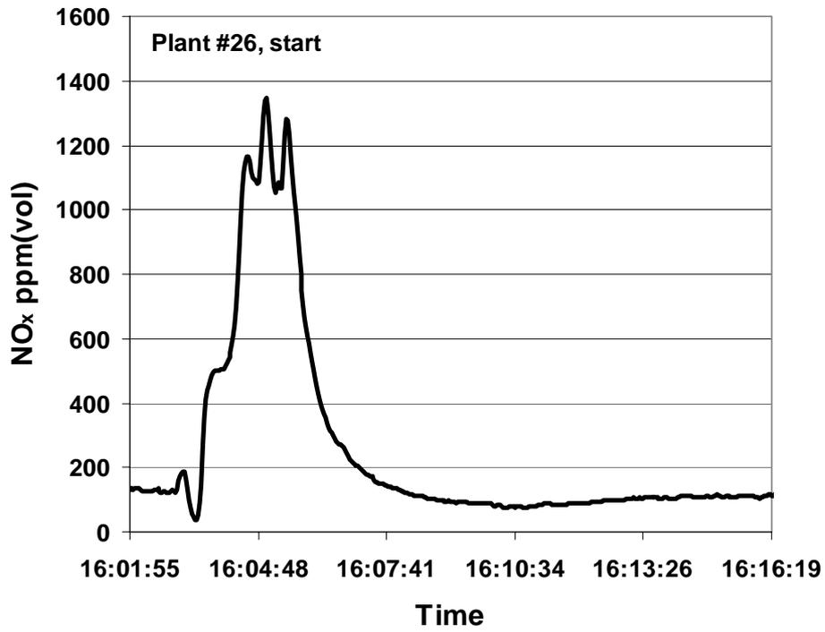
Figure 12 *NO<sub>x</sub> emission for a natural gas engine during start-up*
