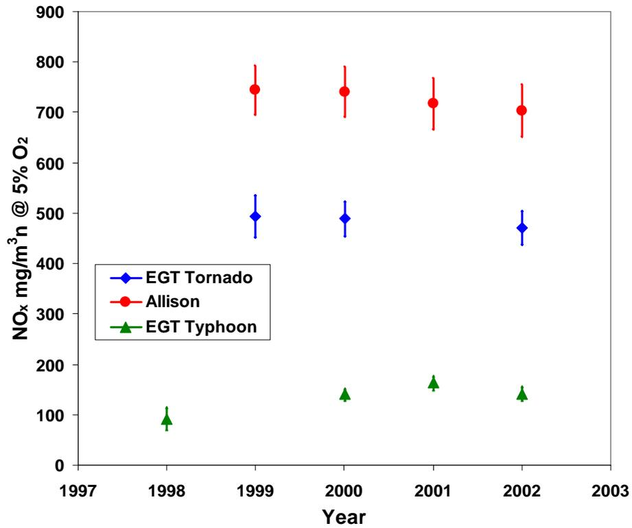
Figure 4 Time series of  $NO_x$  emission data for natural gas turbines. Vertical lines show the uncertainty of the  $NO_x$  measurements.
