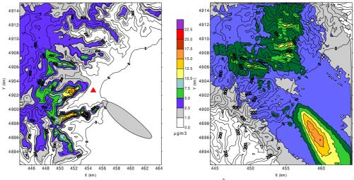
Figure 1. Ground level yearly average concentration of SO<sub>2</sub> ( $\mu$ g/m<sup>3</sup>): (left) ISC3ST, (right) SPRAY driven by MINERVE. The red triangle indicates the emission location.
