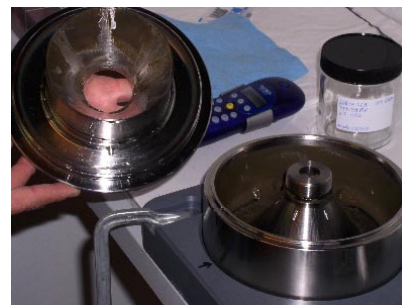
Figur 17.8 < 63 µm-fraktion opsamlet i flow-through centrifugen.
